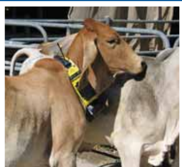
Smart farm: An animal tracking collar with GPS module forms part of a wireless sensor network.
