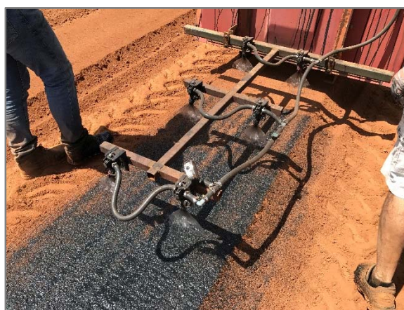
Figure 3: Using multiple spray nozzles to improve uniformity of application (Black pigmented polymer formulation that maintains in-field colouration).
