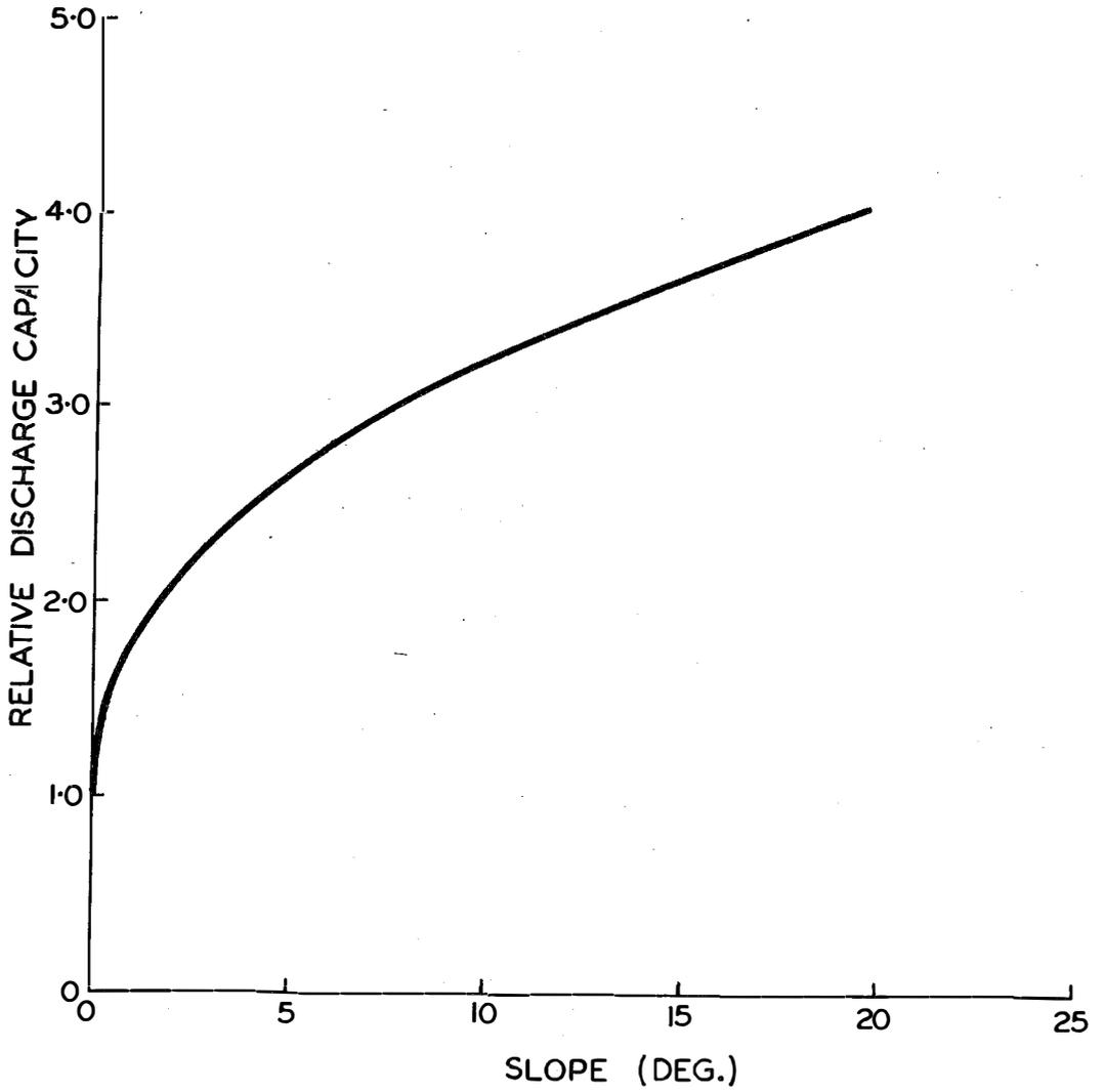
Fig. 4 - Influence of slope on discharge capacity of a drainage channel
