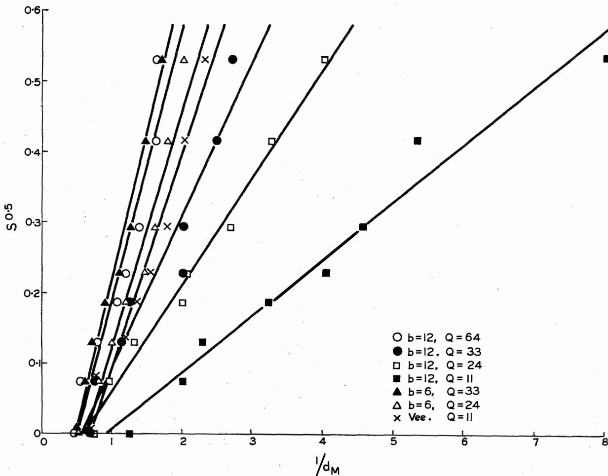
Fig. 3 - Relationship between reciprocal of maximum depth and square root of sine of angle of slope
