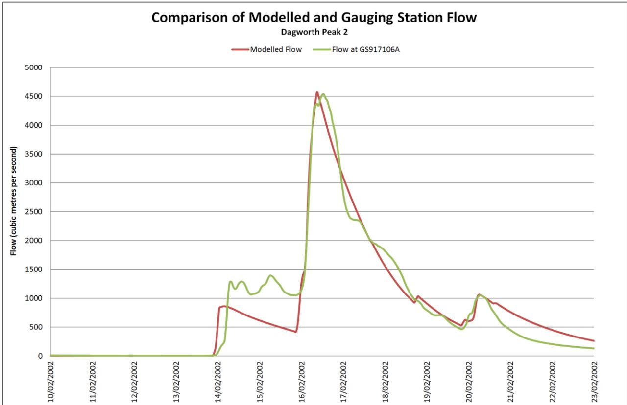
Figure A.1 Comparison of Modelled and Gauging Station Flow for Dagworth Peak 2
