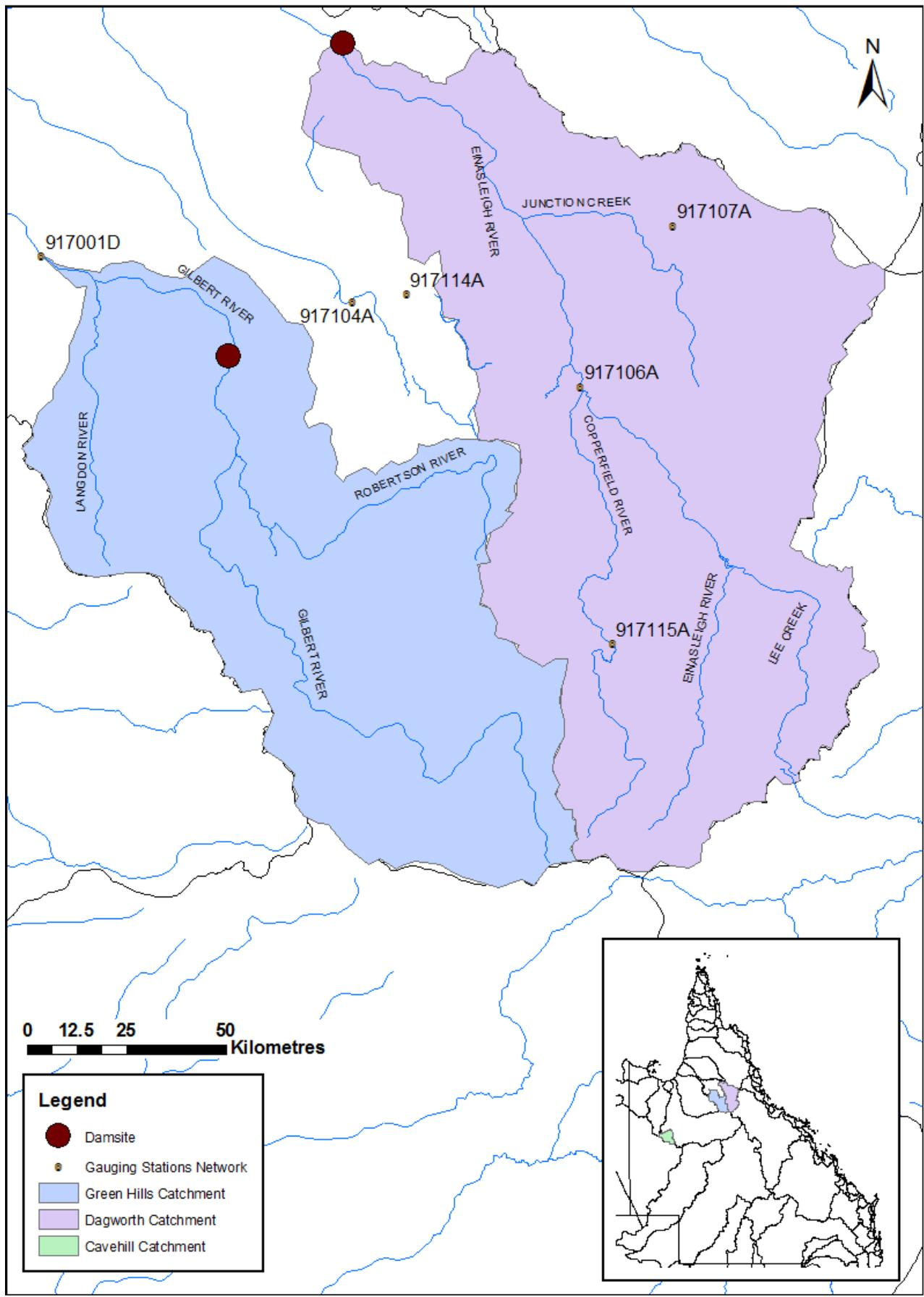
Figure 2.1 Dagworth and Greenhills catchments, streamflow gauging stations and location of potential dam sites
