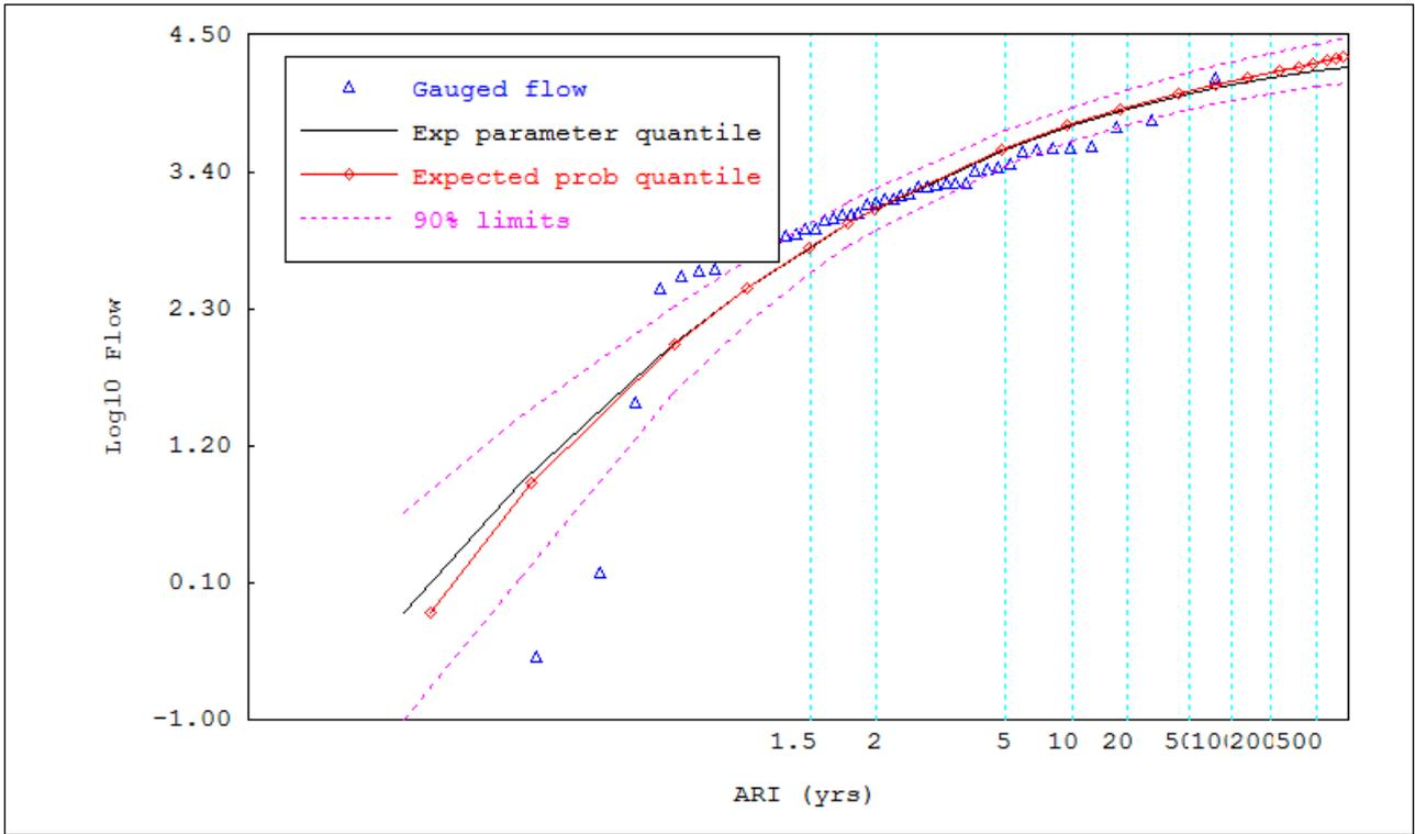
Figure E.2 Greenhills flood frequency plot
