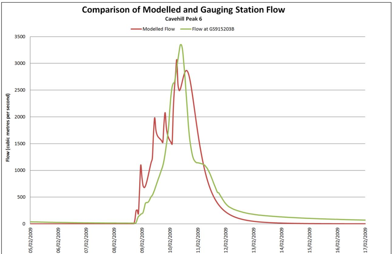
Figure A.7 Comparison of Modelled and Gauging Station Flow for Cavehill Peak 6
