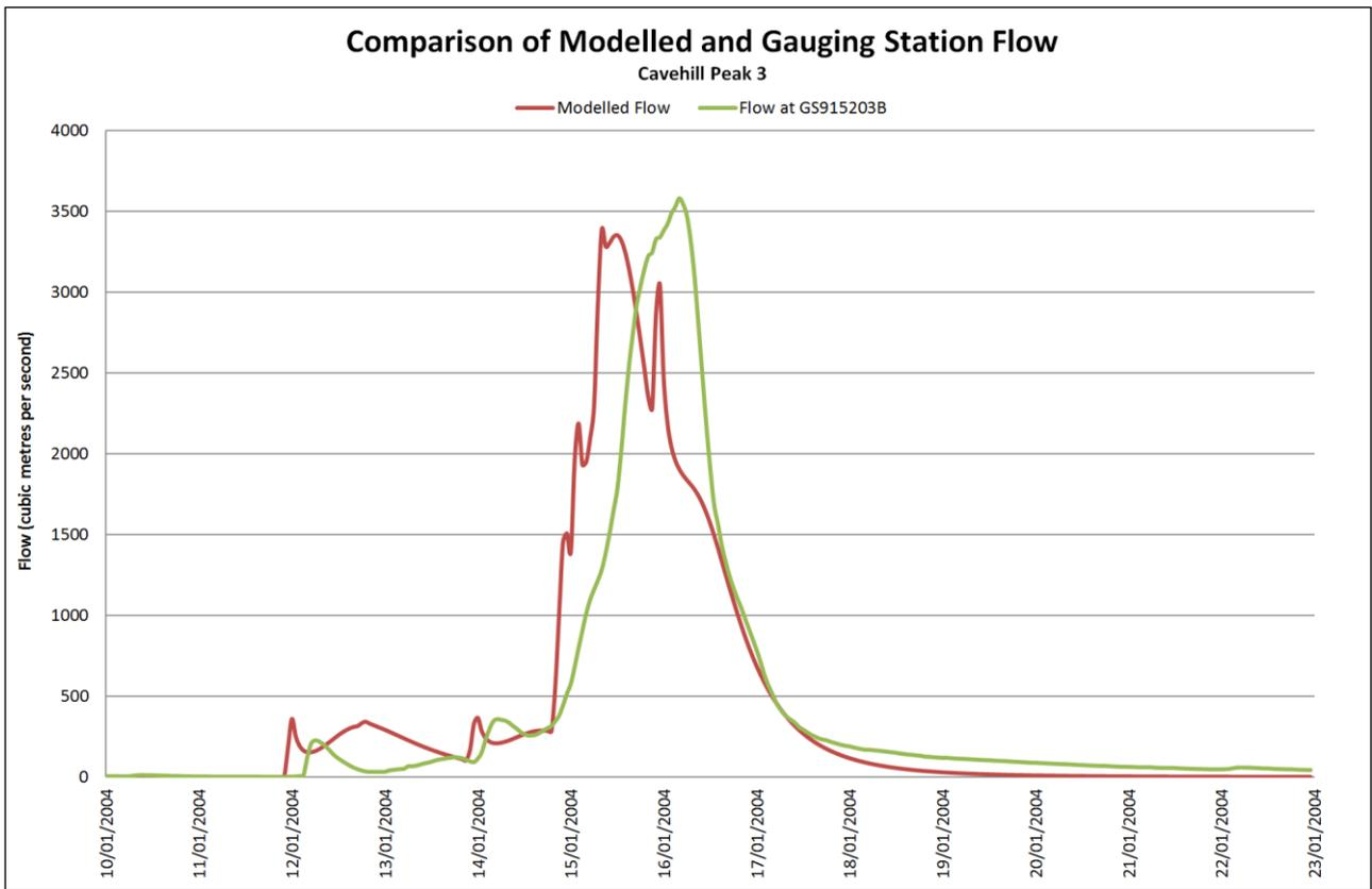
Figure A.6 Comparison of Modelled and Gauging Station Flow for Cavehill Peak 3
