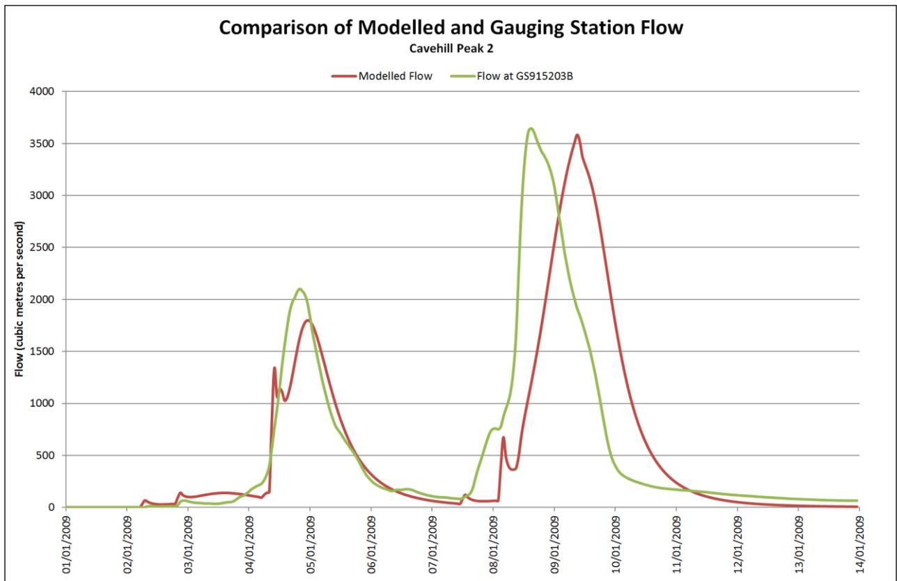
Figure A.5 Comparison of Modelled and Gauging Station Flow for Cavehill Peak 2
