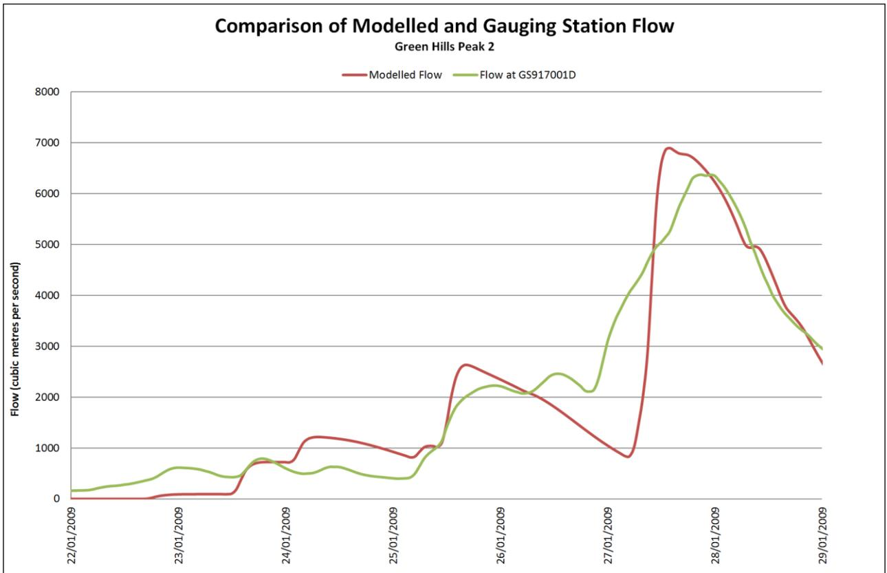
Figure A.3 Comparison of Modelled and Gauging Station Flow for Greenhills Peak 2
