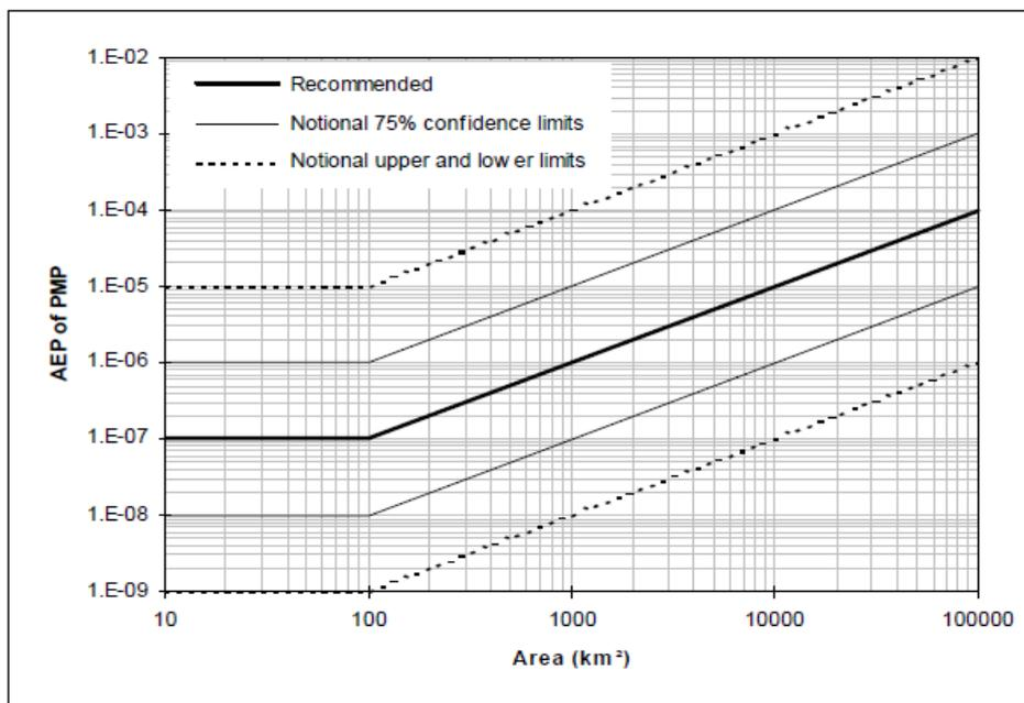
Figure 6.1 Plot to determine the AEP of the PMP based on catchment area (IEAust 1998)
