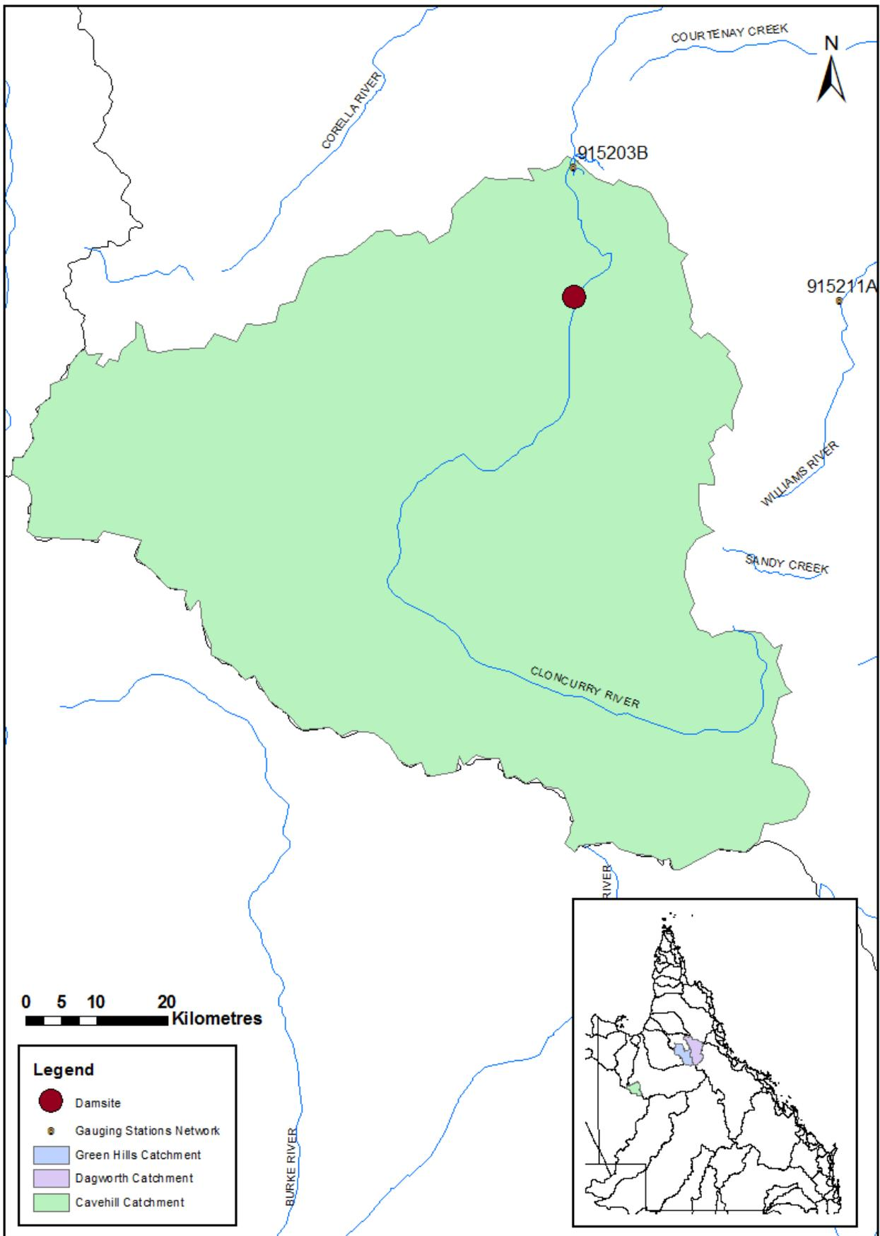
Figure 2.2 Cavehill catchment area, streamflow gauging station and location of potential dam site
