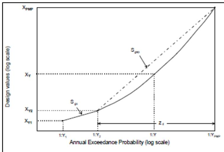
Figure 6.2 Equation and plot demonstrating the interpolation between CRC-FORGE and PMP design rainfall (IEAust 1998)
