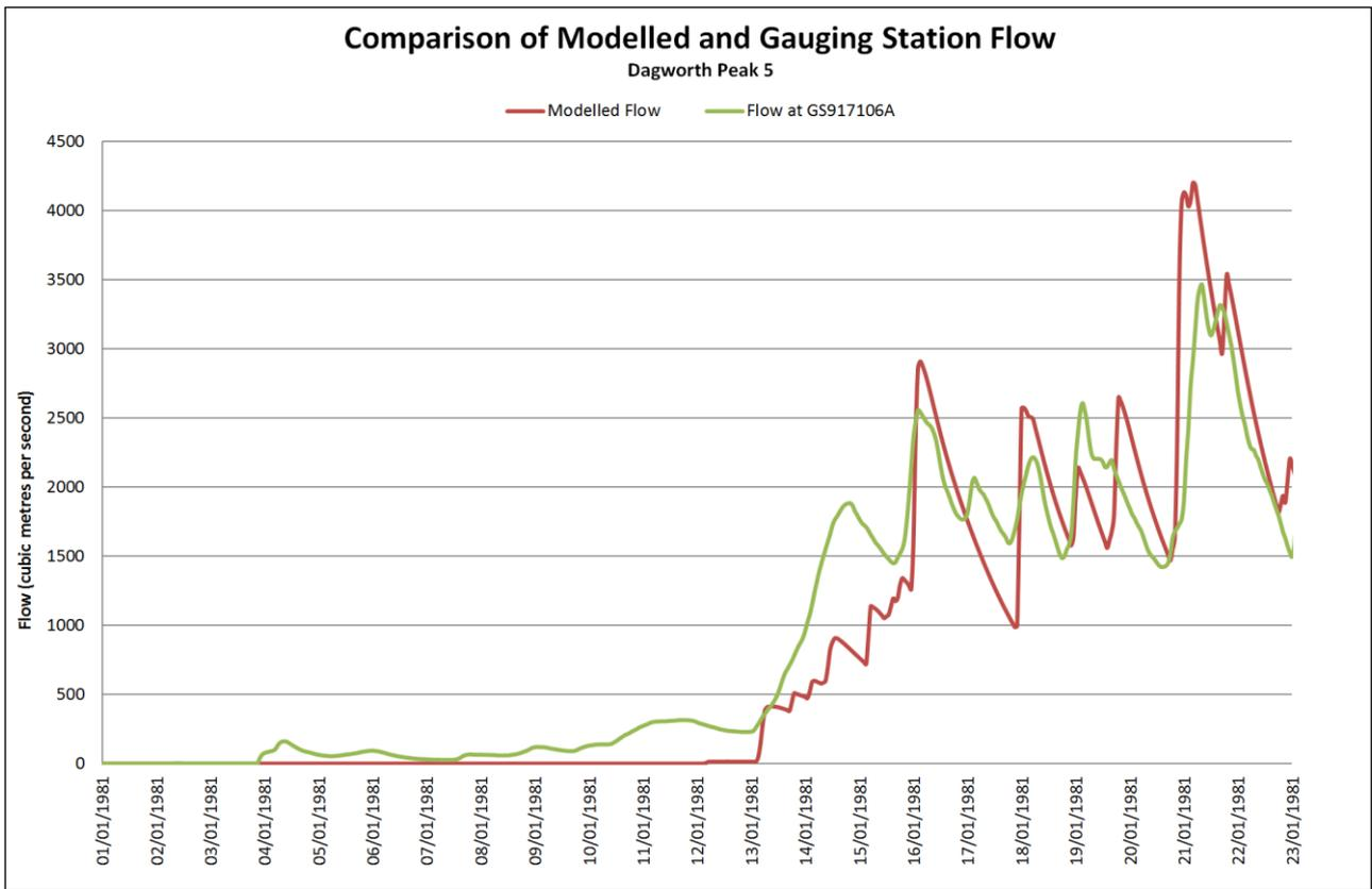
Figure A.2 Comparison of Modelled and Gauging Station Flow for Dagworth Peak 5
