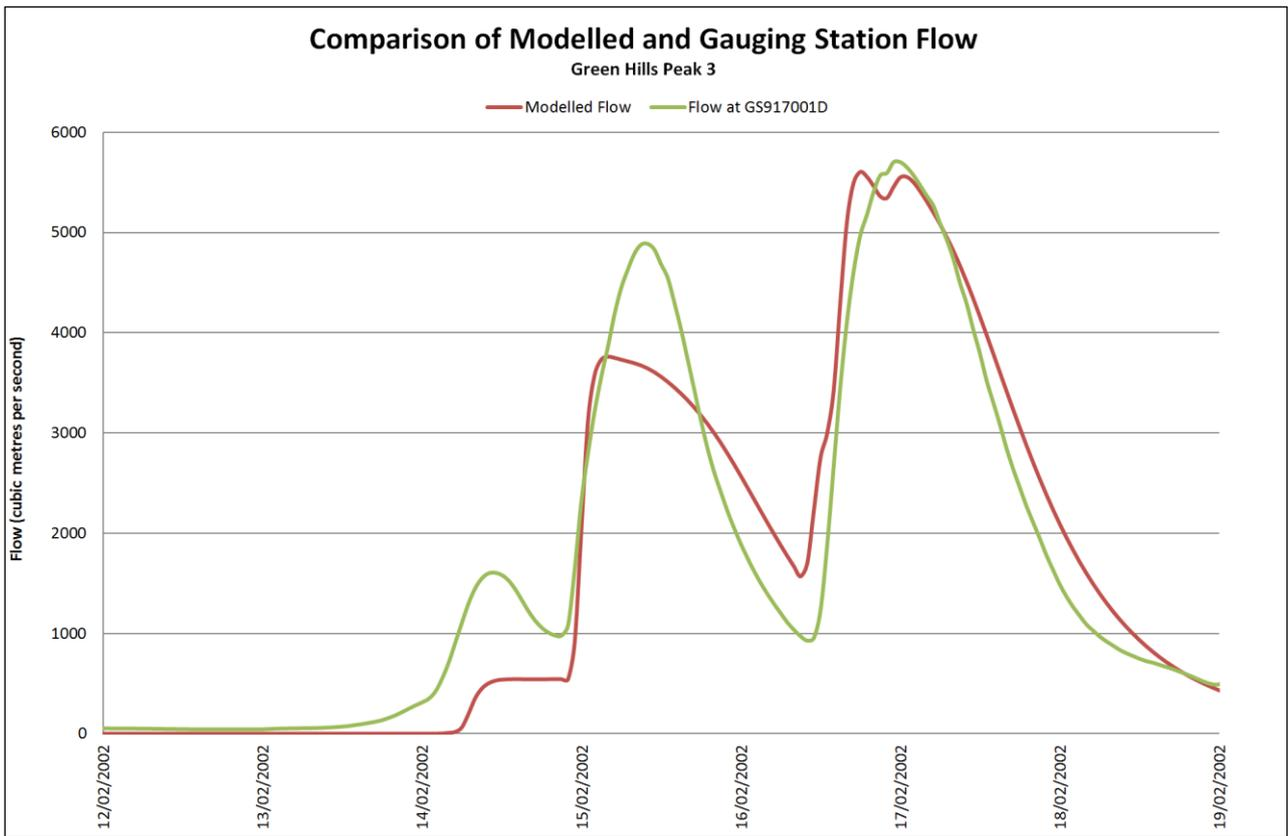
Figure A.4 Comparison of Modelled and Gauging Station Flow for Greenhills Peak 3
