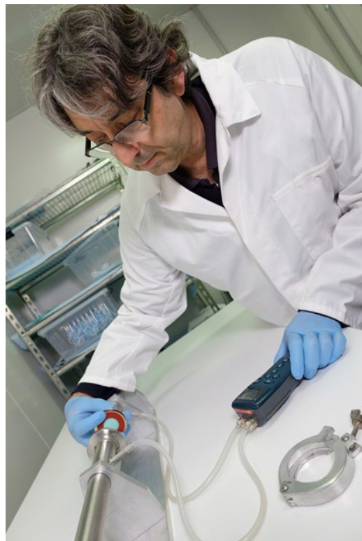
A scientist conducts a Pressure Differential (pressure drop) test to assess breathability by measuring the differential pressure across a mask.
