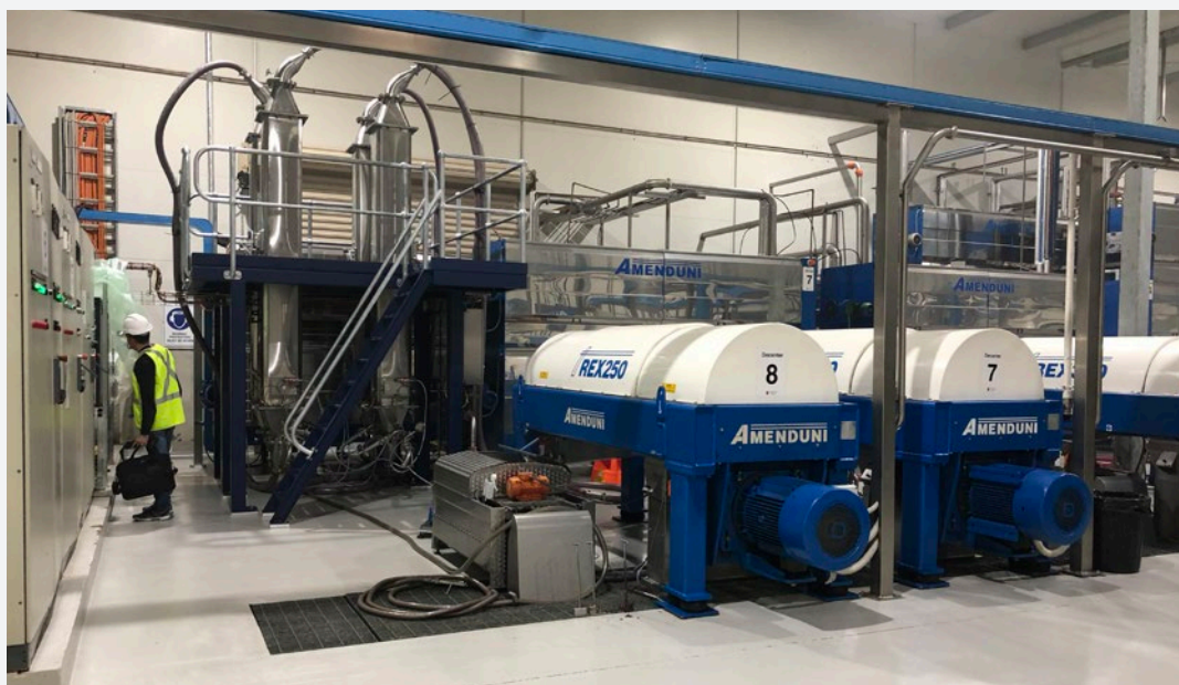
Industrial 3 tonnes per hour Megasonics demonstration olive oil extraction.
