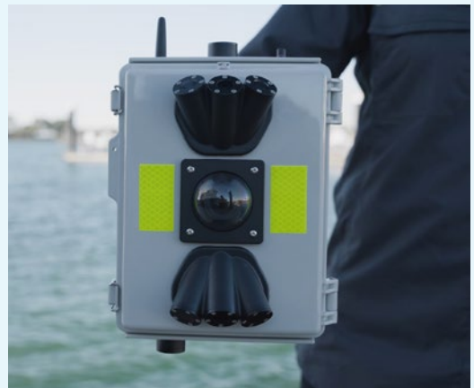
CSIRO's HydraSpectra sensor for installation at the AquaWatch pilot site at Keppel Bay on Darumbal Sea Country, monitoring sediment and dissolved carbon flow from the Fitzroy River towards the Southern Great Barrier Reef.
