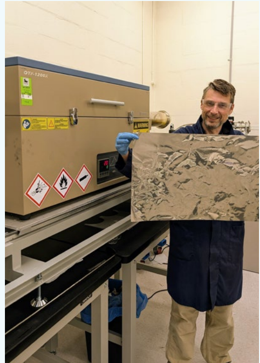
Dr James Cooper, CSIRO Research Scientist, with a GraphAir film synthesised using the scaled chemical vapour deposition (CVD) production process.
