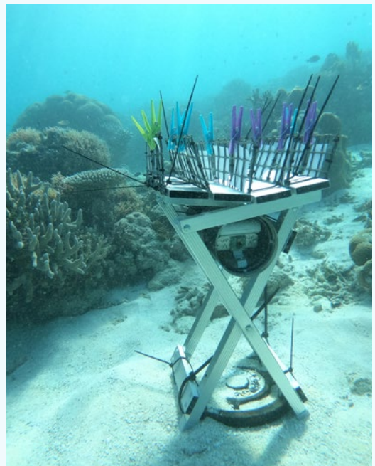
CSIRO researchers invented a novel low-tech way to collect eDNA, making it easier to measure fish species and ocean biodiversity. This photo shows an experiment to test the capacity of different materials to capture eDNA at Ashmore Reef off north Western Australia.
