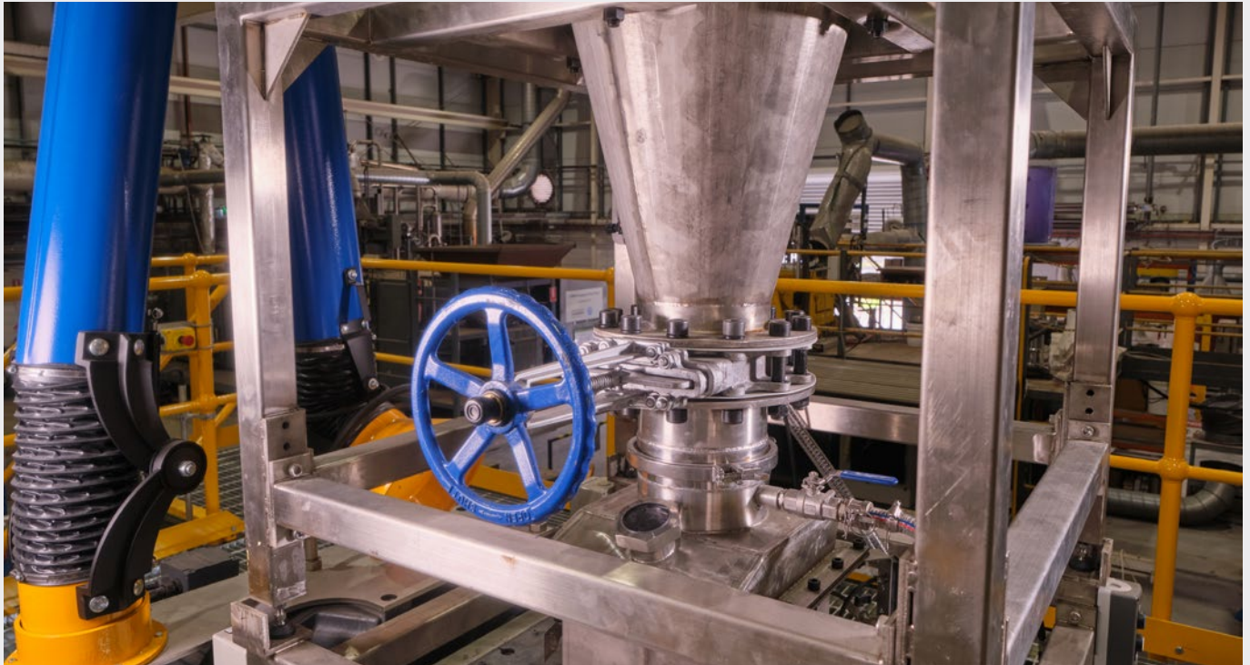
One-of-a-kind CSIRO designed rig for safe shredding of end-of-life Lithium-ion batteries in Clayton Victoria.
