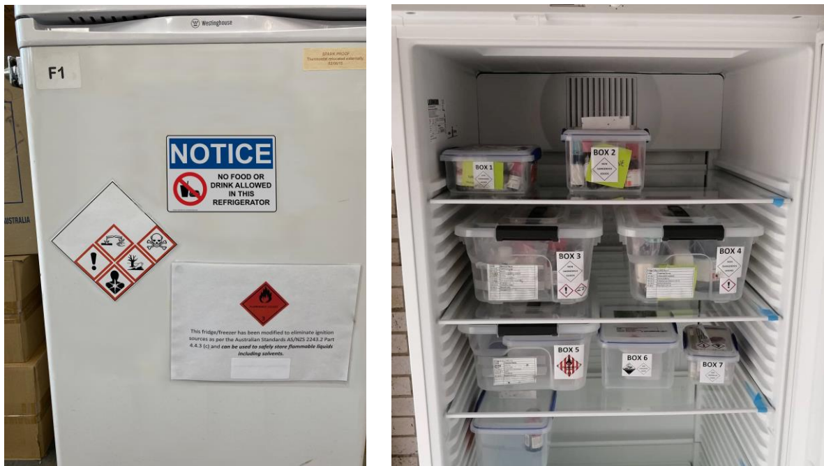
Figure 2. Examples of using a refrigerator to store chemicals.
