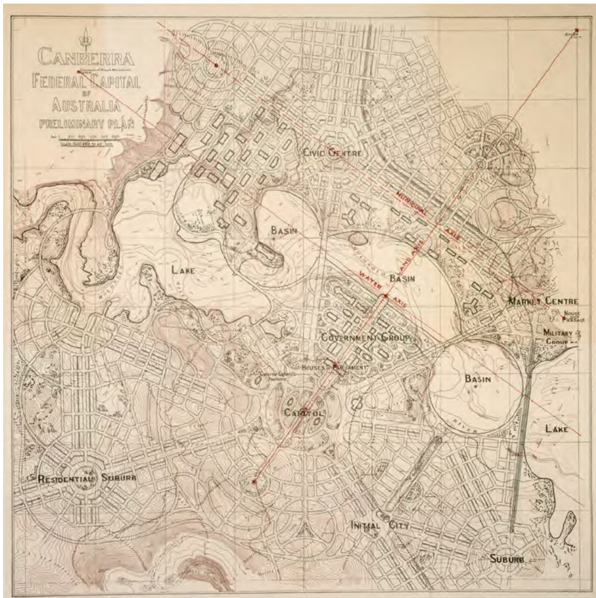
Figure 2.1 The Griffins' plan of design for the federal capital showing land, water and municipal axes, 1911. The three formal basins of the city centre and their flanking lakes are especially clear in this plan. (Source: NAA, A1, 1917/7242)
