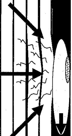
Cracking above UCG cavity
