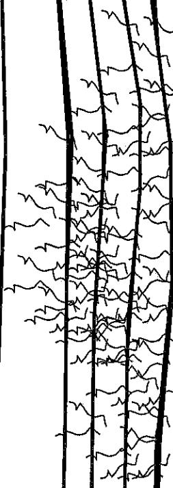
Roof collapse into UCG cavity
