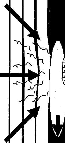
Cracking above UCG cavity
