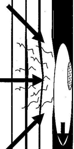
Cracking above UCG cavity
