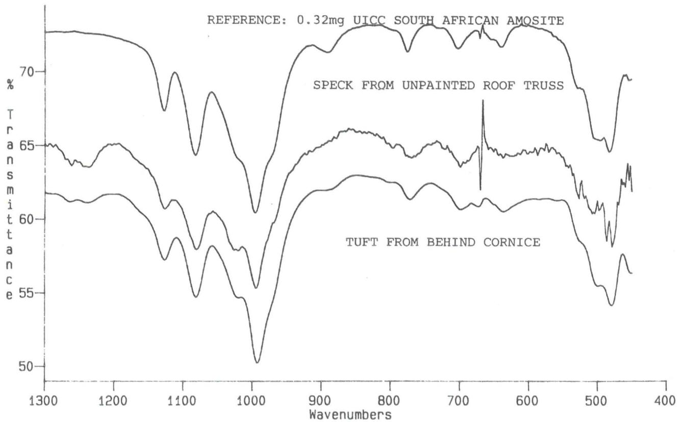
Figure 4. Specks of asbestos fluff residue on unsealed underside of roof truss and infrared spectra of residues from Program removal sites.
