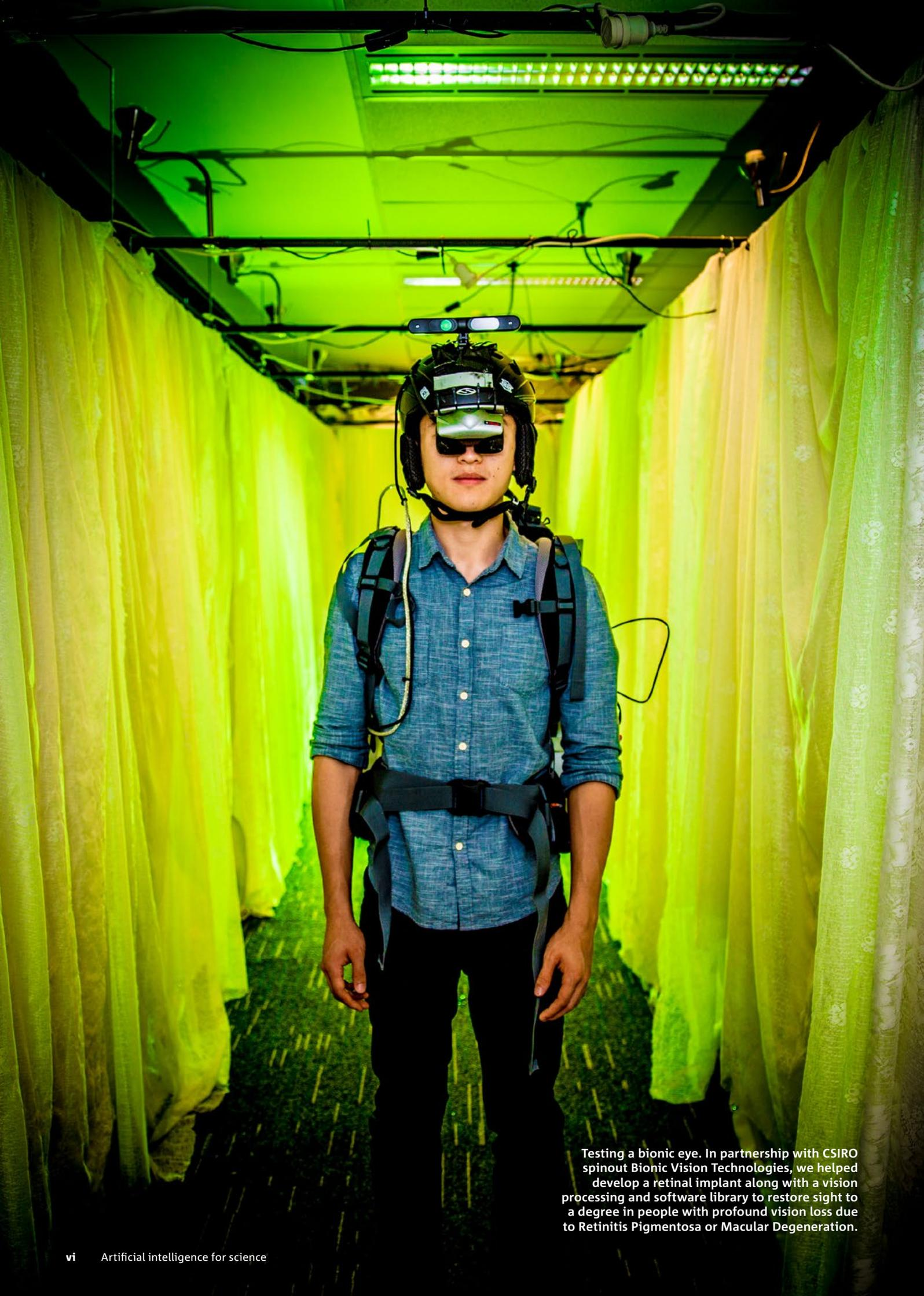
Testing a bionic eye. In partnership with CSIRO spinout Bionic Vision Technologies, we helped develop a retinal implant along with a vision processing and software library to restore sight to a degree in people with profound vision loss due to Retinitis Pigmentosa or Macular Degeneration.
