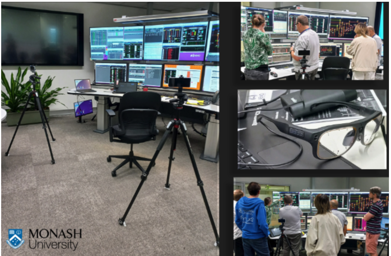
Figure 5: illustrating the data collection day, showing 2-way tripod video camera set up for recording the screens as the operators sat at the workstation (left), the Tobii Pro glasses v3 used for the eye tracking recording (right middle) and the researcher team discussing and observing components of the screen right (upper and lower).
