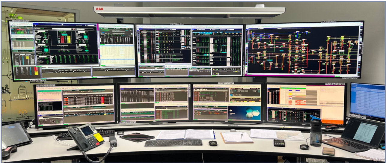
Figure 1: One operator's workstation at AEMO in the training environment. Each workstation has the same seven-screen set up. In addition, each has a keyboard, mouse, a telephone and a smaller screen (see right above laptop). Some operators also have access to a laptop and/or tablet. In the training room there is a second phone as one is the training phone, the other is used if the room is converted to a live control room.
