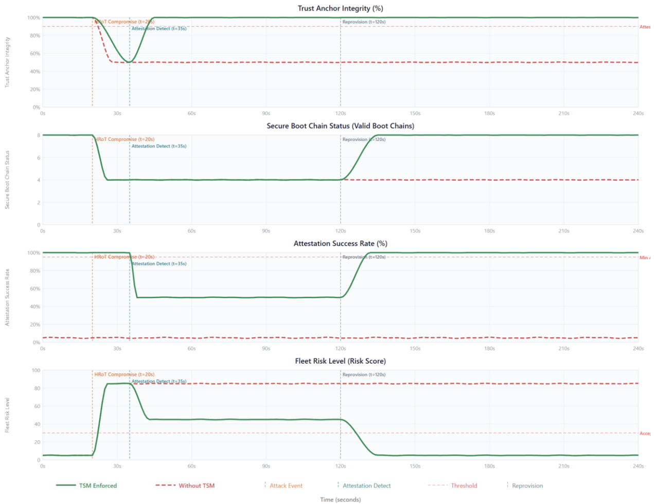
Figure 44: TC4: Trust anchor compromise. The TSM-enabled enforcement provides remote attestation capabilities to detect HRoT manipulation using attestation cycle and detection latency to isolate the promised EVSE chargers from the fleets and restore EVSE fleet.
