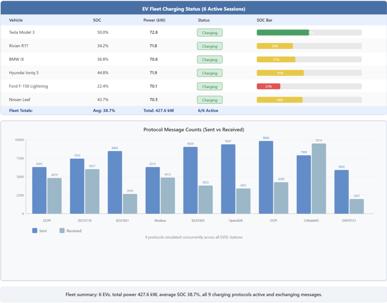
Figure 38: Layer 2 results: EV fleet charging profiles and statistics of communication protocols interactions
