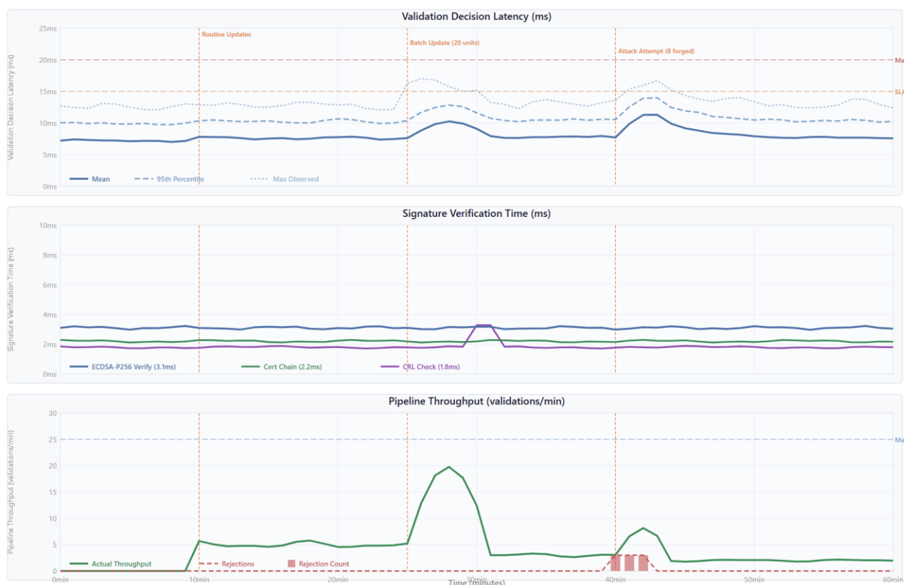
Figure 48: The aggregate performance of the TSM firmware update security pipeline for the 60-minute simulation window. The mean latency is 7.6 ms indicate the operational feasibility and latency acceptance of TSM enforcement policies for the firmware update.
