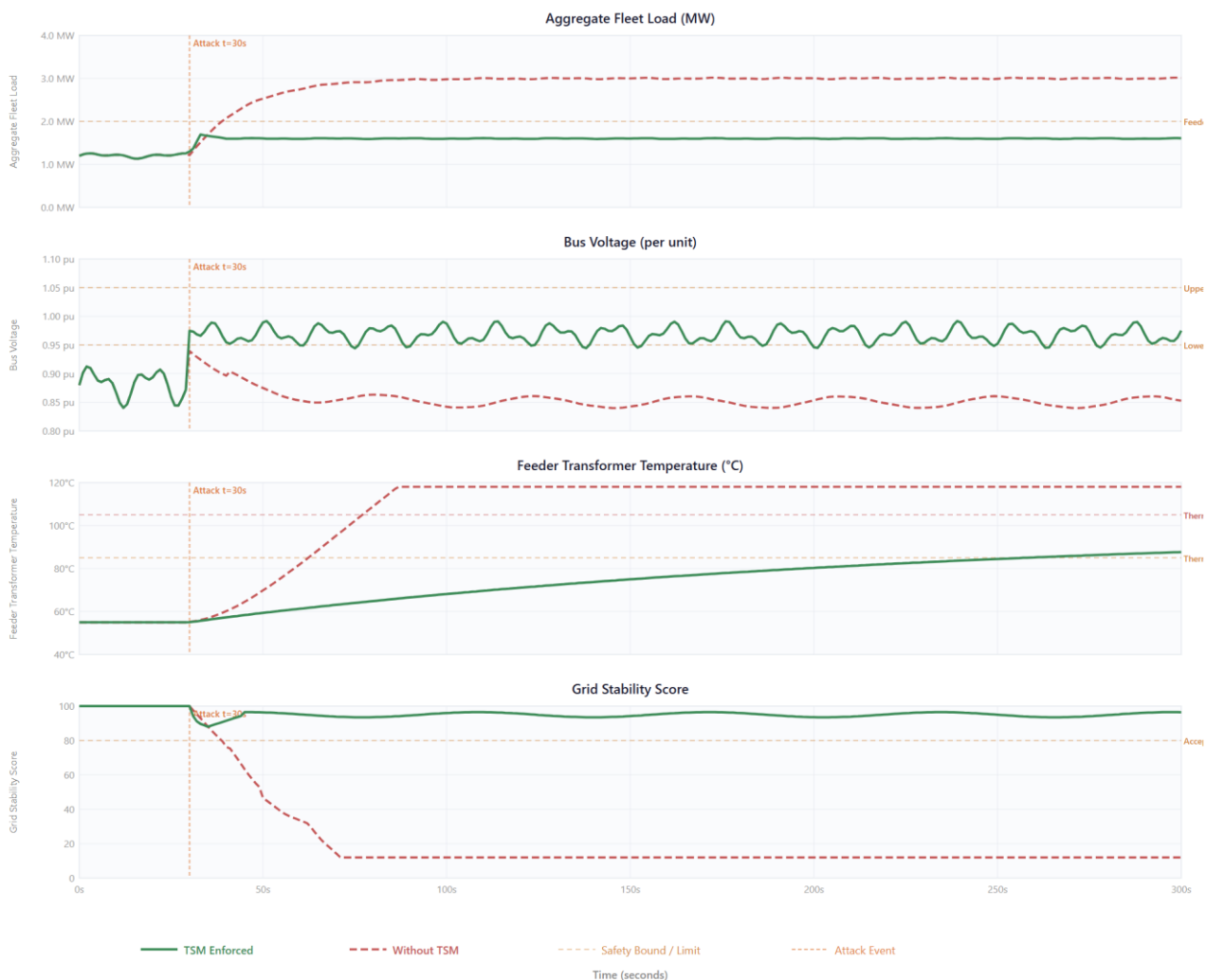
Figure 45: A fleet-level coordinated load attack occurs under TC2 when a malicious firmware update is initiated simultaneously on 20 EVSE chargers. This causes the total load to surge to 3.0 MW, exceeding the distribution feeder's rated capacity by 150%. With TSM
