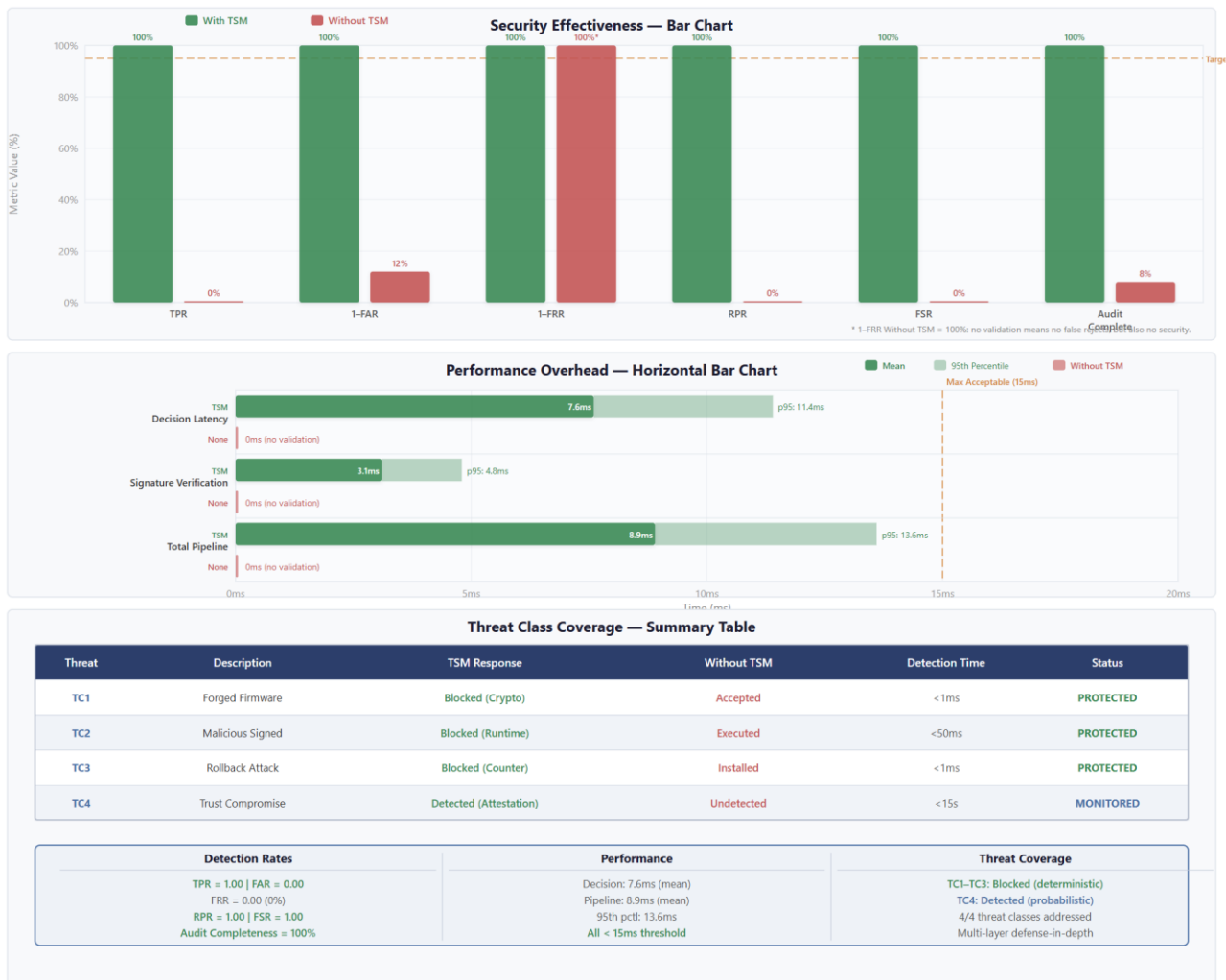
Figure 47: The summarized TSM-enabled security metrics are: True Positive Rejection Rate (TPR) = 1.00, False Accept Rate (FAR) = 0.00, False Reject Rate (FRR) = 0.00, and Fail-Safe Reliability (FSR) = 1.00. All firmware update-related threat classes are mitigated.
