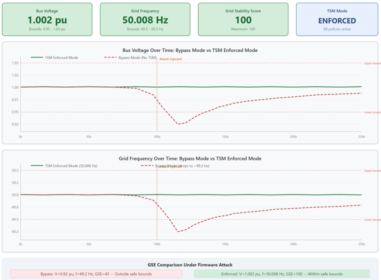
Figure 40: Layer 3 results: TSM enforced frequency and voltage stability of power grid.
