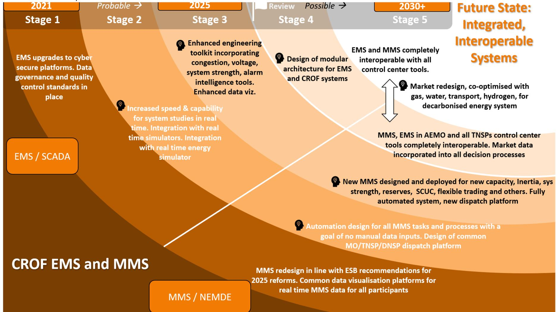
Figure 4-4 CROF Roadmap for EMS / SCADA and MMS / NEMDE
