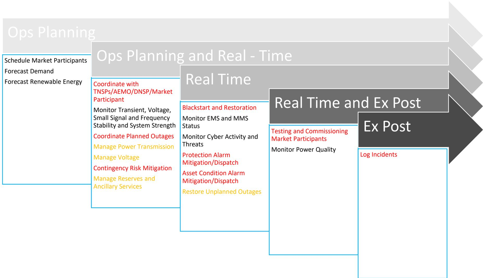
Figure 3-4 Graphical interpretation of time frame of processes. Red are processes which are mostly manual, Orange are processes that are manual and/or automatic and black are processes that are mostly automatic
