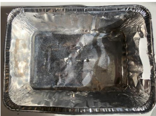
Prepared aluminium tray with three puncture holes in the base to allow groundwater to pass through, and a narrow hole along the short side for runoff to flow.
