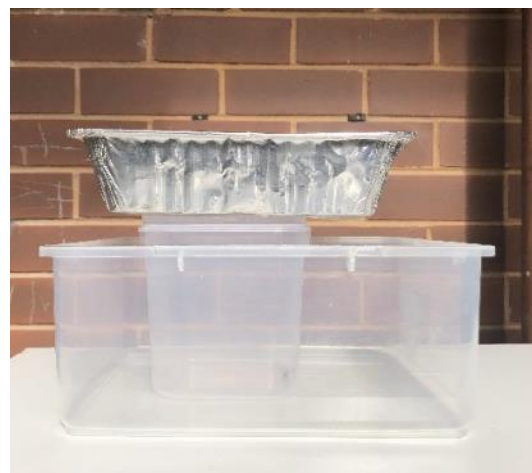
Test Tray 1 set up for testing, with ground water collecting in the smaller container and runoff flowing into the larger, surrounding container.
