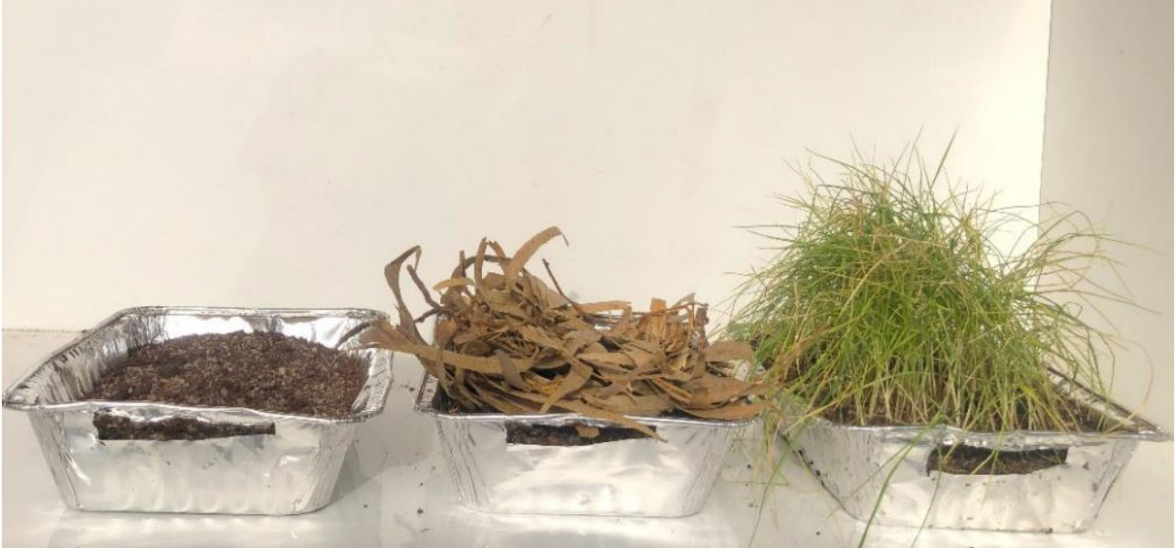
Three trays ready for testing: Tray 1 (left) peat moss and sand mix, Tray 2 (middle) peat moss and sand mix covered with leaf litter, Tray 3 (right) peat moss and sand mix with living wheatgrass.
