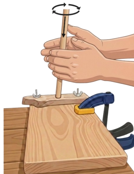
Figure 3 Set-up for hand drill experiment
