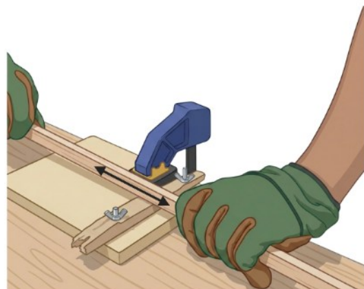
Figure 4 Set-up for fire saw experiment
