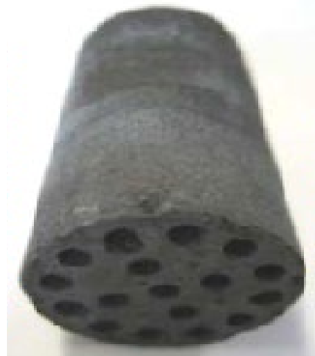
Fabricated (HMCFC) length: 80mm, diameter: 30mm, number of channels: 17
