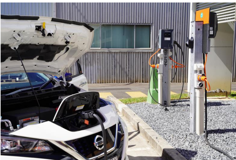
Figure 5 - CHAdeMO V2G using Nissan Leaf and Quasar Wallbox DC charger
