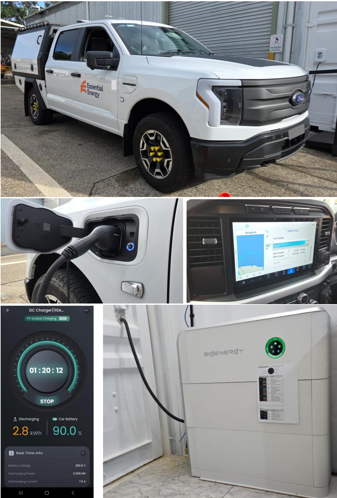
Figure 6 - CCS2 bidirectional charging using AUSEV Ford F-150 Lightning and Sigenergy DC charger.
