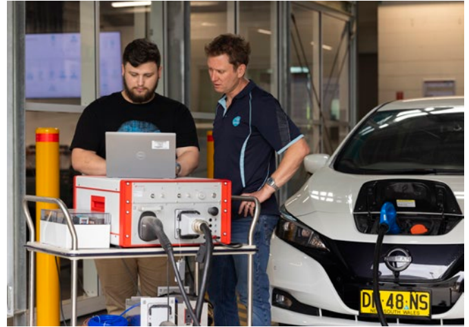
Engineers configuring the Electric Vehicle Supply Equipment (EVSE) emulator for a Vehicle-to-Home (V2H) experiment.
