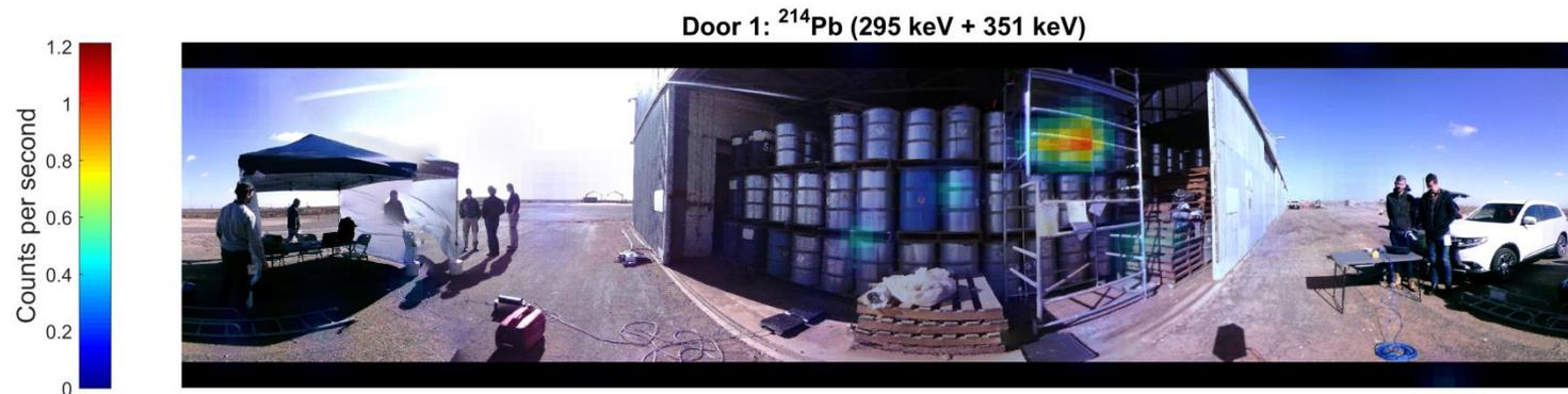
Figure 4: Gamma image from  $^{214}\text{Pb}$  (295 keV + 351 keV peaks) at Location 1. The total dose rate at this location was  $0.3 \mu\text{SV/h}$ , which is approximately equivalent to  $1.5 \times$  the average background dose rate in Australia, or 10% of the dose rate on an international flight.
