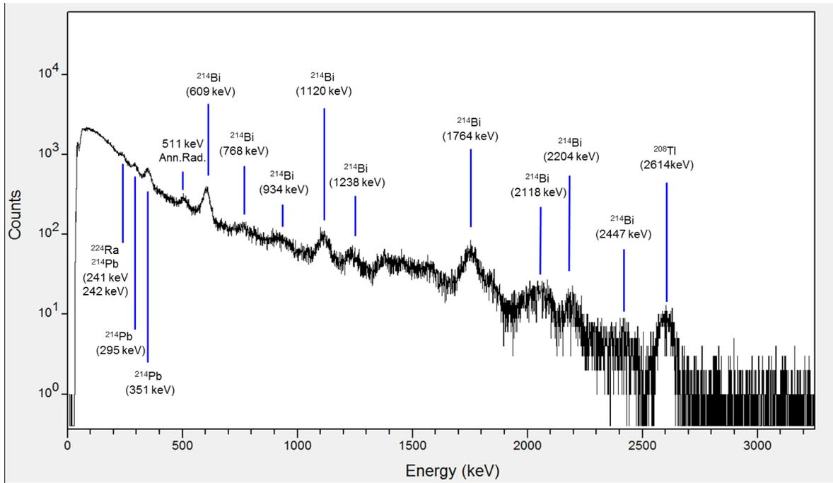
Figure A1: Gamma spectrum from Location 1 (256 minutes total acquisition)
