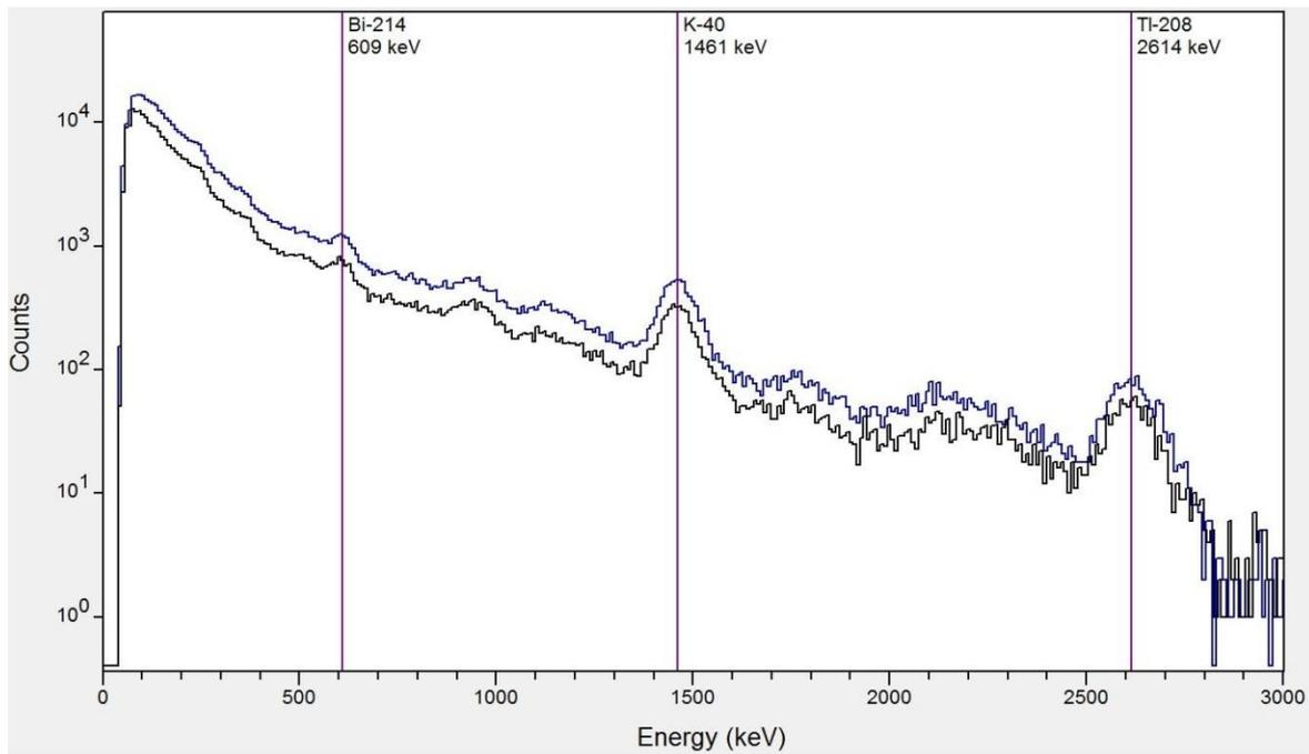
Figure A6. Background gamma ray spectrum acquired on the north east side of the hangar (black line) and the Eldo Hotel carpark (blue line). 1200 s total acquisition per spectra. Note the spectra in this figure were recorded with a different detector than the one used for Figures A1-A5. As such, direct comparison of count rates is not meaningful.
