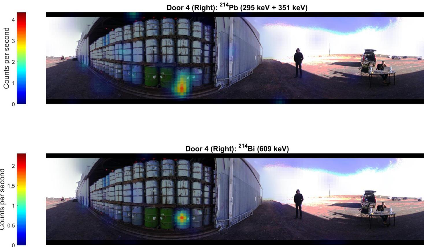
Figure 7: Gamma images from (top)  $^{214}\text{Pb}$  (295 keV + 351 keV peaks) and (bottom)  $^{214}\text{Bi}$  (609 keV peak) at Location 4. The total dose rate at this location was  $0.6 \mu\text{SV/h}$ , which is approximately equivalent to  $3 \times$  the average background dose rate in Australia, or 20% of the dose rate on an international flight.
