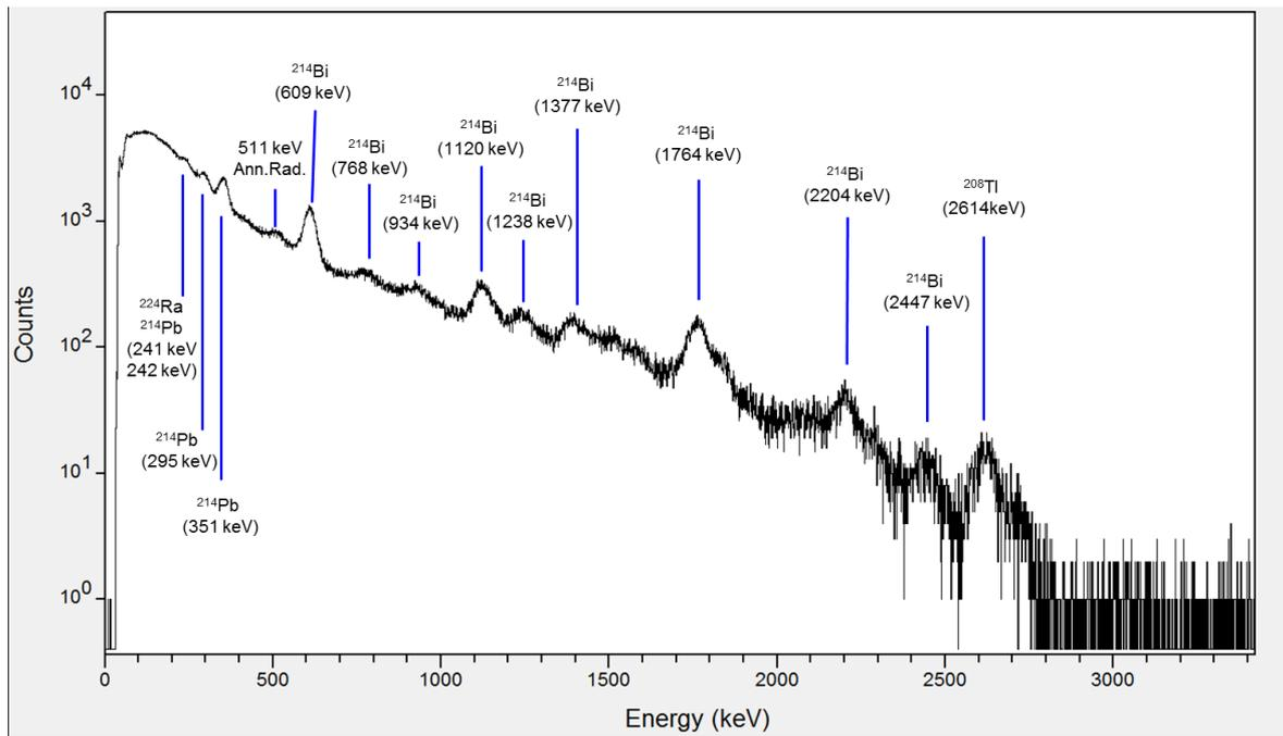
Figure A5: Gamma spectrum from Location 5 (205 minutes total acquisition)
