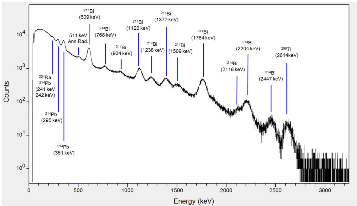
Figure A3: Gamma spectrum from Location 3 (183 minutes total acquisition)
