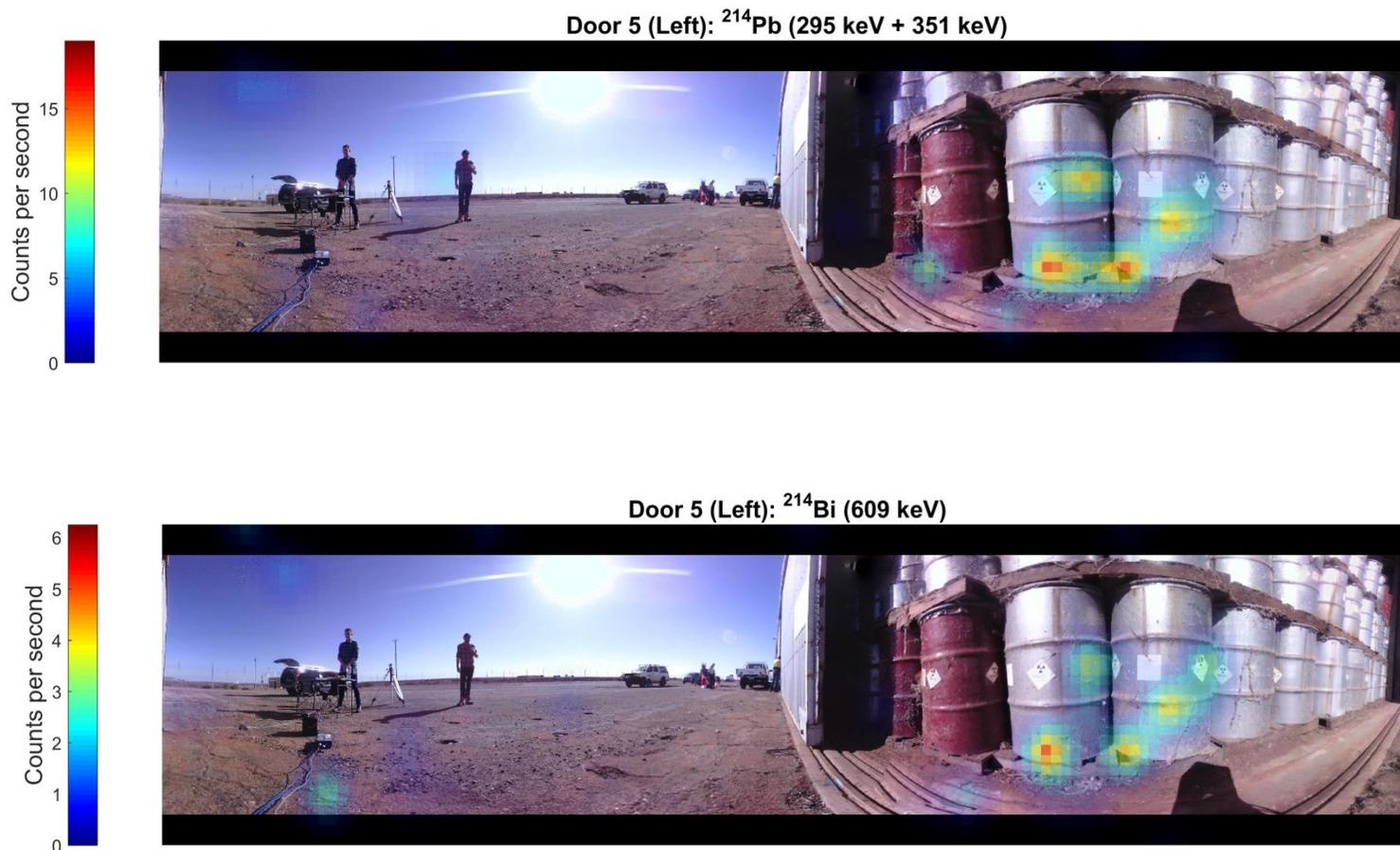
Figure 6: Gamma images from (top)  $^{214}\text{Pb}$  (295 keV + 351 keV peaks) and (bottom)  $^{214}\text{Bi}$  (609 keV peak) at Location 3. The total dose rate at this location was  $3 \mu\text{SV/h}$ , which is approximately equivalent to the dose rate on an international flight. NB The dose rate at this location is higher as the camera is very close to the drums,  $\sim 85 \text{ cm}$ , to allow for higher resolution imaging.
