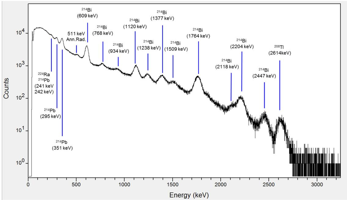
Figure 3: Gamma spectrum recorded at Location 3 (Bay 5, NE side). The spectrum is dominated by peaks originating from the <sup>238</sup>U decay series daughters, <sup>214</sup>Bi and <sup>214</sup>Pb.
