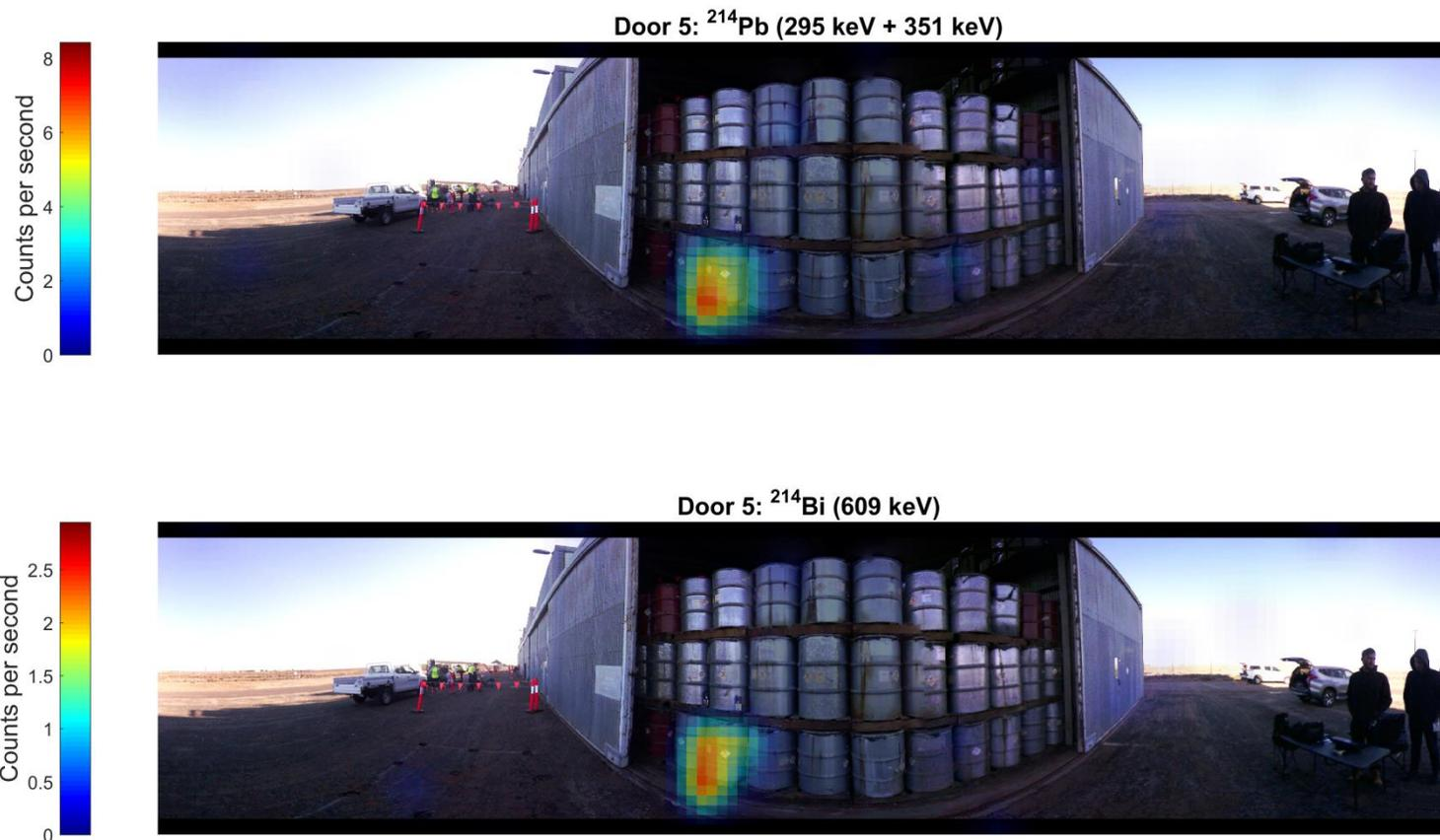
Figure 5: Gamma images from (top)  $^{214}\text{Pb}$  (295 keV + 351 keV peaks) and (bottom)  $^{214}\text{Bi}$  (609 keV peak) at Location 2. The total dose rate at this location was  $0.3 \mu\text{SV/h}$ , which is approximately equivalent to  $1.5 \times$  the average background dose rate in Australia, or 10% of the dose rate on an international flight.
