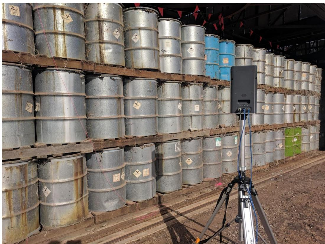
Figure 2: Photos of the Cyclops gamma imaging system deployed at Woomera; (Top) Location 2, (Bottom) Location 5, as listed in Table 1.
