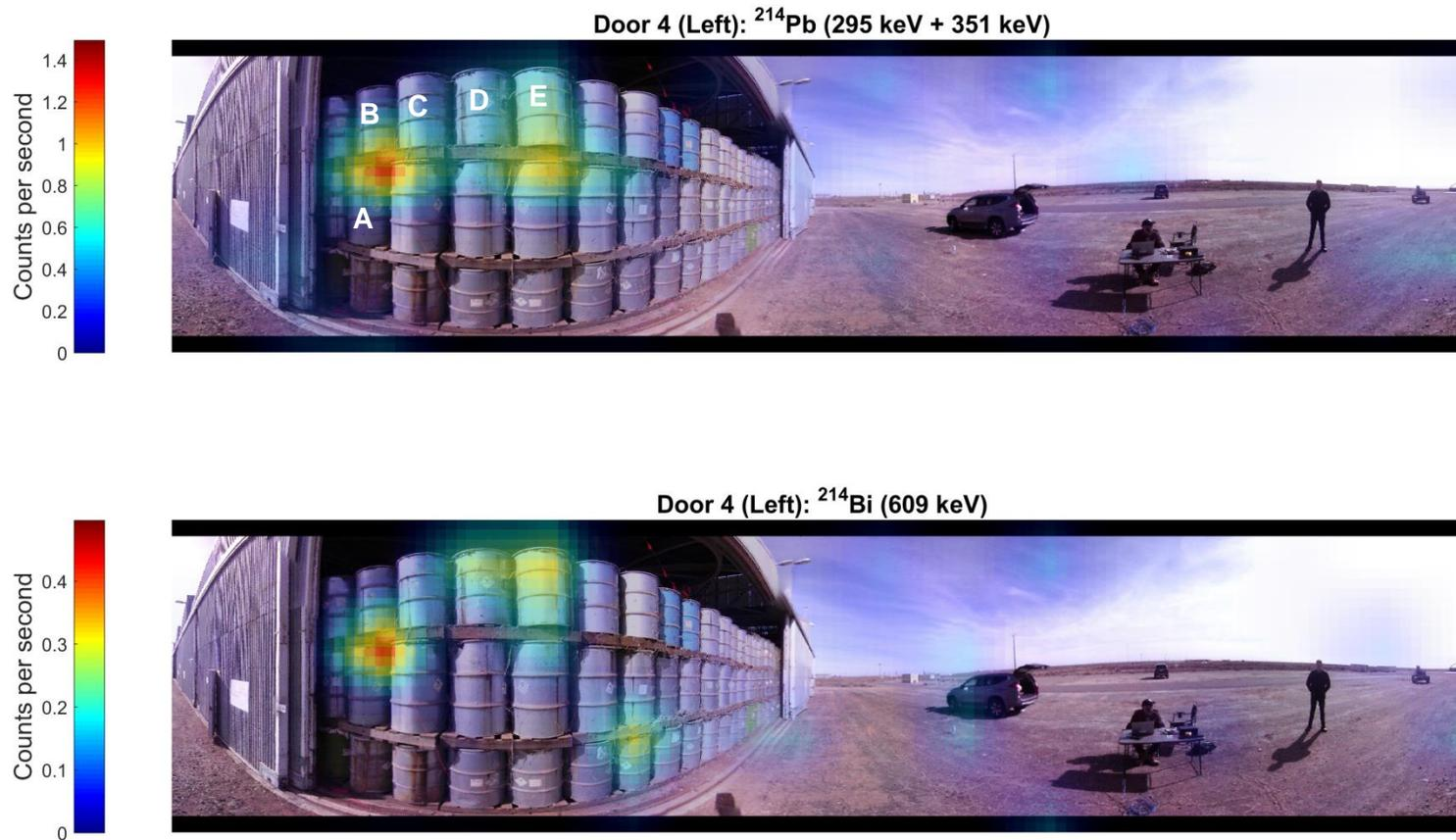
Figure 8: Gamma images from (top)  $^{214}\text{Pb}$  (295 keV + 351 keV peaks) and (bottom)  $^{214}\text{Bi}$  (609 keV peak) at Location 5. The total dose rate at this location was  $0.5 \mu\text{SV/h}$ , which is approximately equivalent to  $2.5 \times$  the average background dose rate in Australia, or 17% of the dose rate on an international flight.
