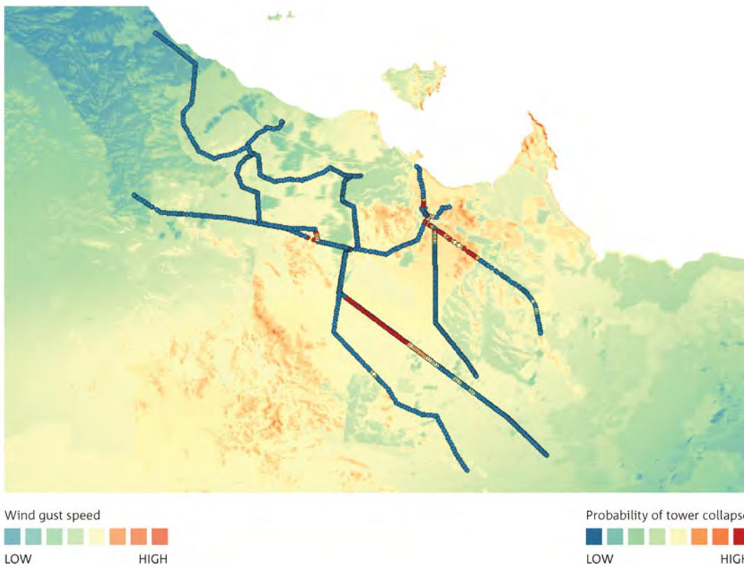
**Figure 28** Impact results for a selected scenario event showing local gust wind speed and the probability of tower collapse across the transmission system.
