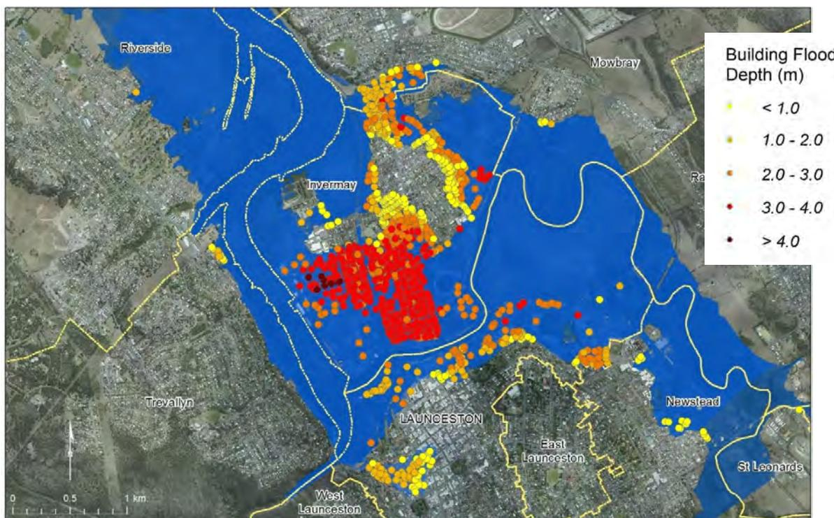
Figure 27 Launceston inundation depth above ground floor for 1000 year annual recurrence interval flood provided by Geosciences Australia from their systems
