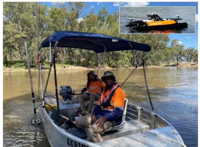
Researchers use sonar equipment from boats like this, including remote controlled boats (inset), to collect accurate information about cross sections of the river network (known as river bathymetry) to inform their hydrodynamic modelling. This image, from geospatial experts AAM, pictures AAM personnel using sonar equipment on the water.
