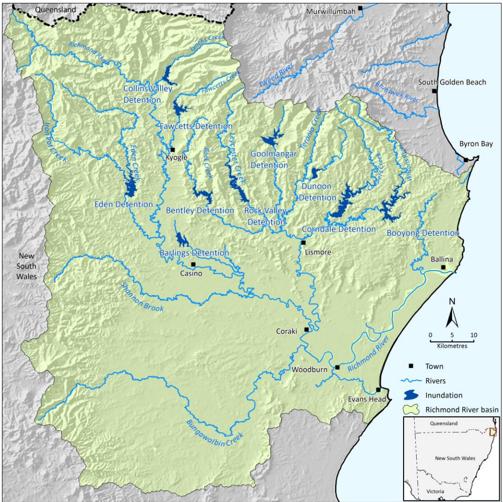
Figure 11 Aerial view of all completely full detention storages in Bundle 2 across the Richmond River catchment.
