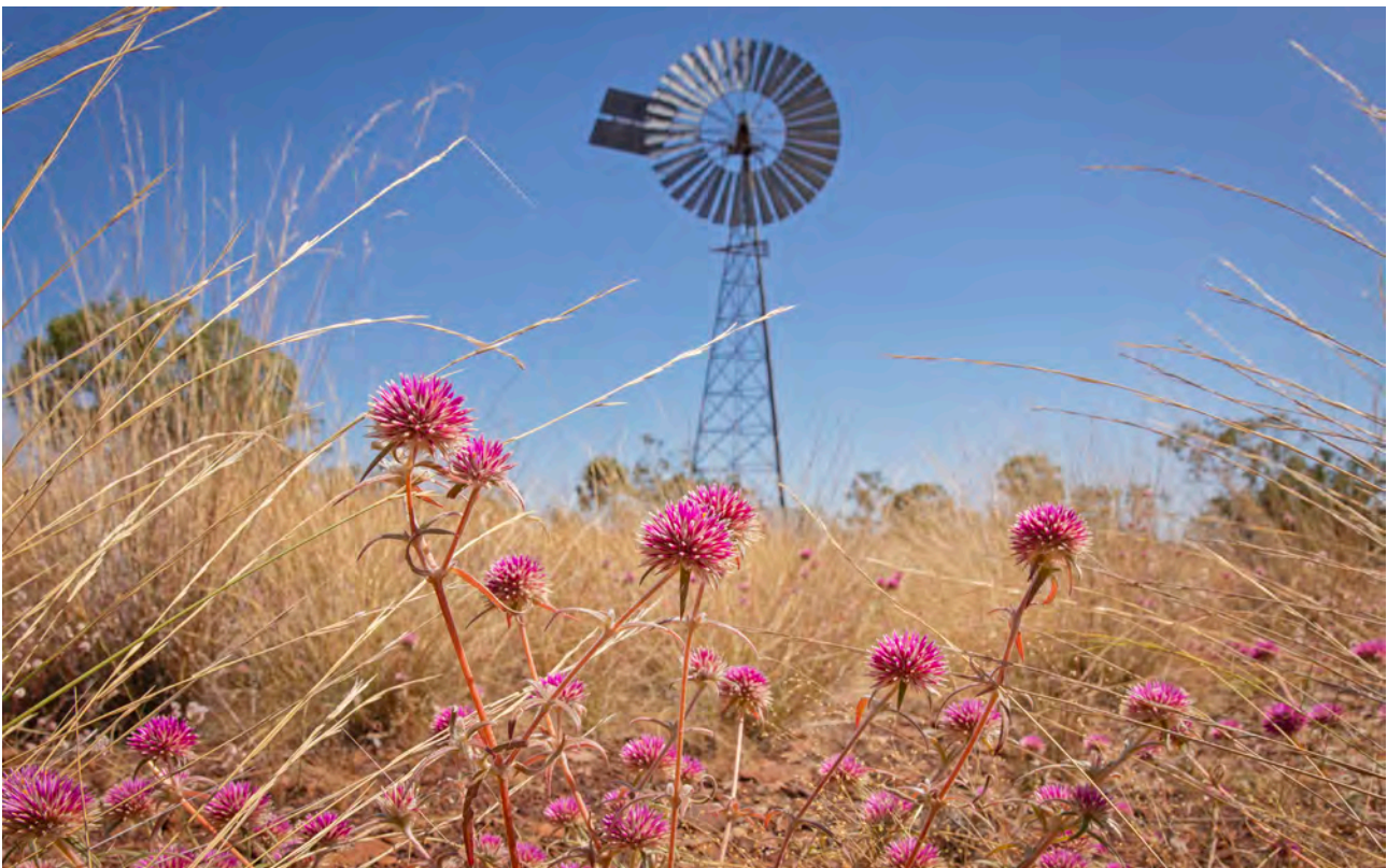
Figure 5-4 Groundwater pumps powered by the wind provide water points for cattle
