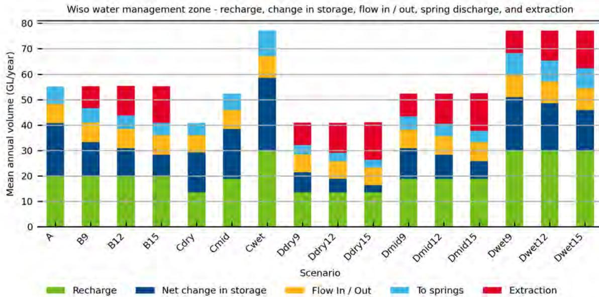
Figure 6-2 Main components of the mean annual water balance for the Wiso Water Management Zone representative of 2060 conditions (2055 to 2065)
