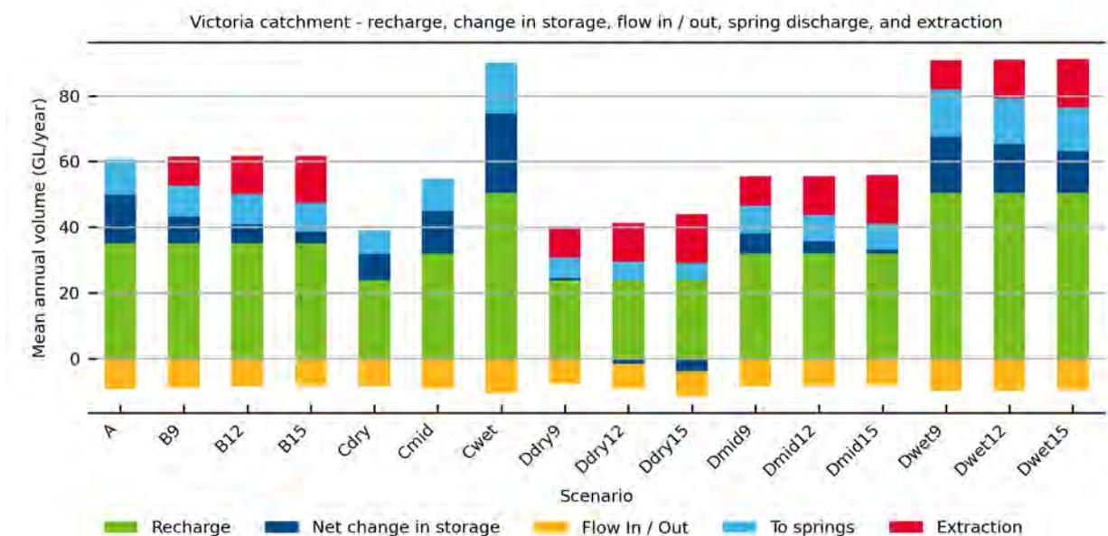
Figure 6-1 Main components of the mean annual water balance for the Victoria catchment representative of 2060 conditions (2055 to 2065)
