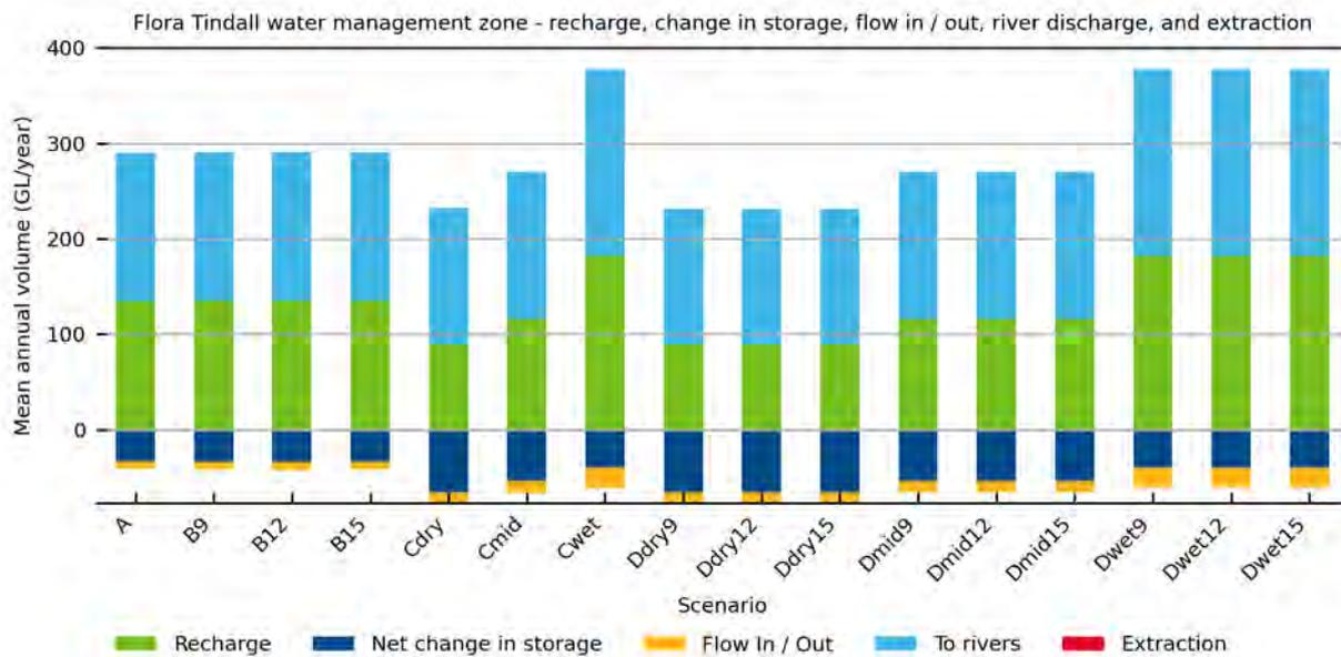
Figure 6-3 Main components of the mean annual water balance for the Flora Tindall Water Management Zone representative of 2060 conditions (2055 to 2065)
