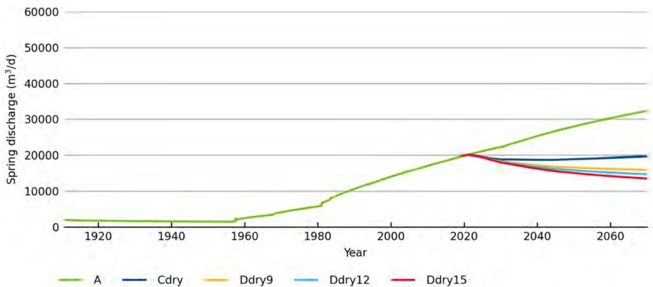
**Figure 5-18 Groundwater discharge to springs and evapotranspiration under scenarios A, Cdry, Ddry9, Ddry12 and Ddry15**
