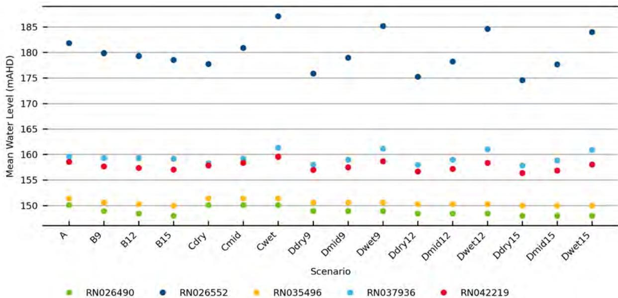
Figure 6-5 Mean groundwater level for the period from 2055 to 2065 under all scenarios for sites RN026490, RN026552, RN035496, RN037936 and RN042219
