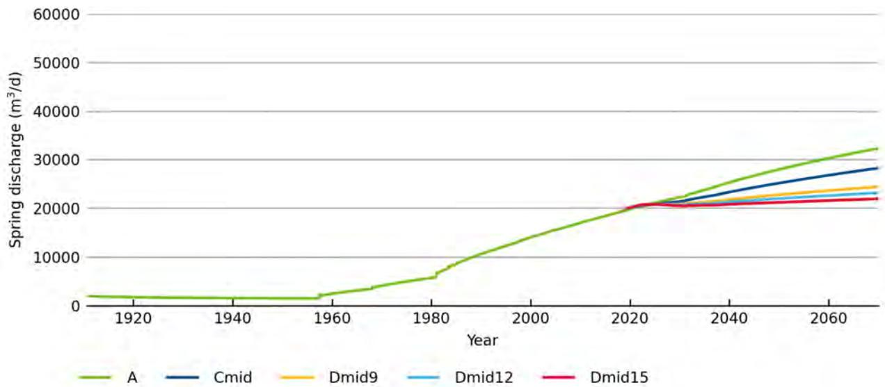
Figure 5-19 Groundwater discharge to springs and evapotranspiration under scenarios A, Cmid, Dmid9, Dmid12 and Dmid15
