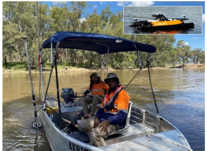
Researchers will use sonar equipment from boats like this, including remote controlled boats (inset), to collect accurate information about cross sections of the river network (known as river bathymetry) to inform their hydrodynamic modelling. This image, from geospatial experts AAM, pictures AAM personnel using sonar equipment on the water.
