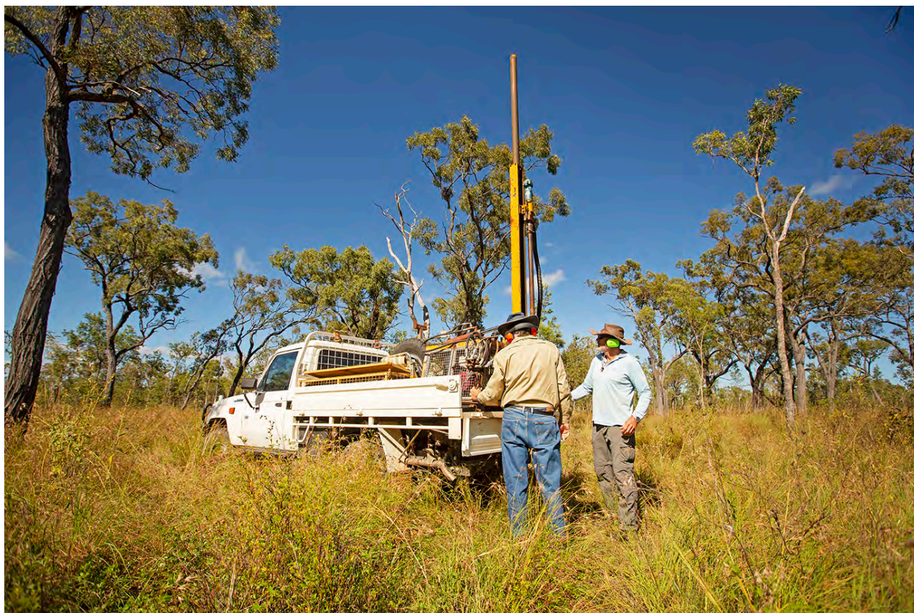
Figure 4-2 Collecting soil cores in the field using a vehicle-mounted push core rig. The collected soil will be analysed in the field and a subset subjected to laboratory analysis
