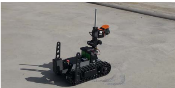
ATLAS robot built to take measurements on top of drums
