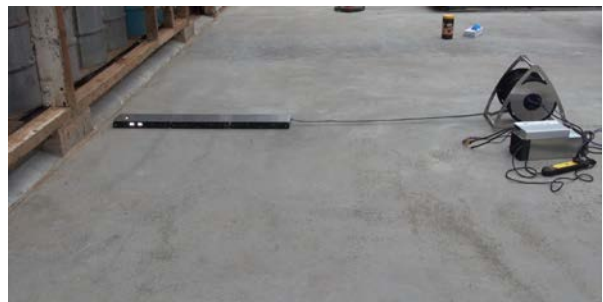
PEABODY robot travelling under drums to take measurements
