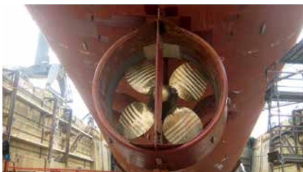
The reconditioned propeller and repaired kort nozzle fitted back on the vessel.
