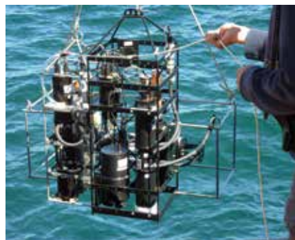
Deploying the optics frame. Credit: Martina Doblin
