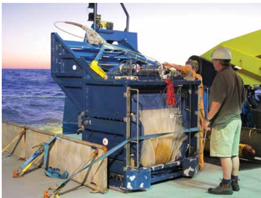
Preparing the EZ Net for deployment. The EZ Net contains up to ten nets that can be opened at different depths and provides real-time telemetry to the vessel whilst deployed. Credit: Megan Saunders
