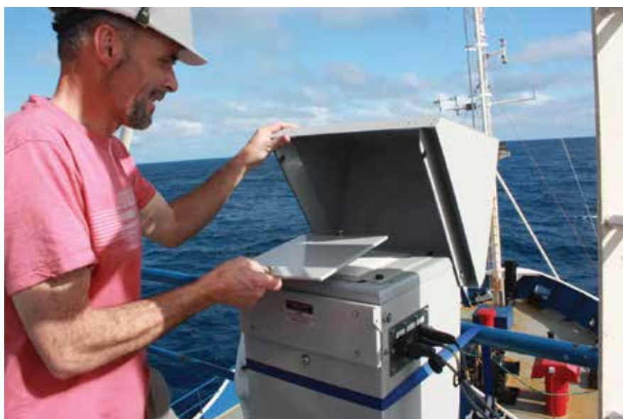
Installation of filter for collection of marine aerosol particles above the bridge. Credit: Laurie Burns
