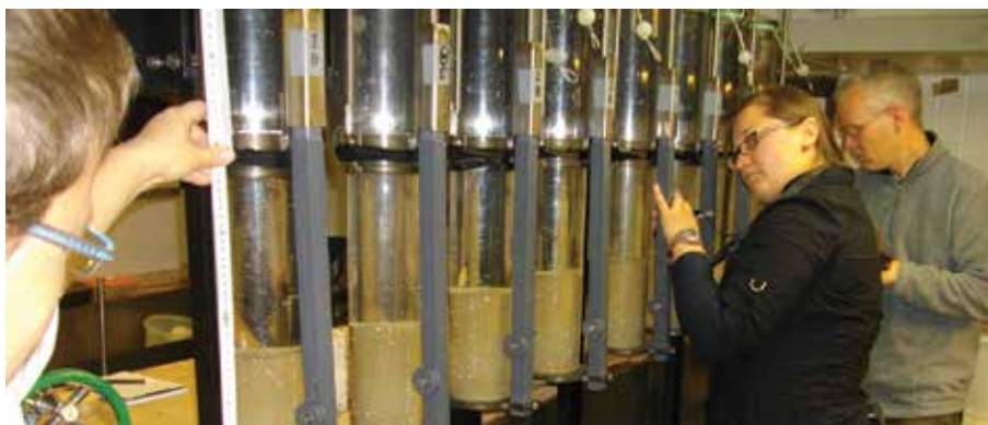
The 8 multitubes containing sediment and water [at the interface] are fixed to a frame in the ship's laboratory for examination and extrusion. Credit: Lyndsay Dean
