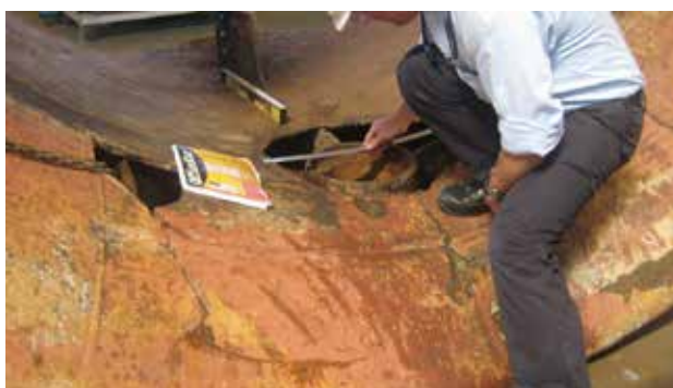
As noted in the underwater inspection the kort nozzle was cracked and in some places metal plating was missing.
