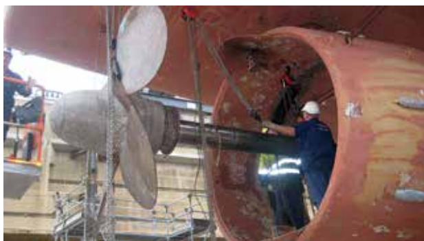
The propeller being removed from the vessel.
