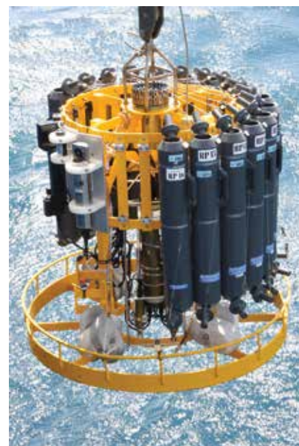
CTD package being lowered into the water.
