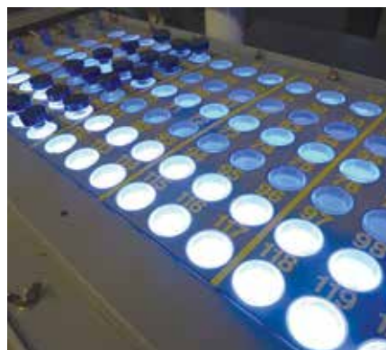
Assessing primary productivity using a photosynthetron. Credit: Martina Doblin
