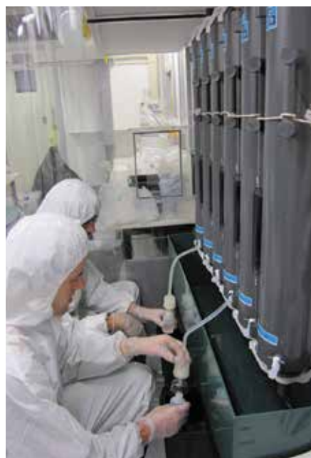
Filtration for micronutrients from the trace metal rosette in a clean air container laboratory. Credit: Andrew Bowie
