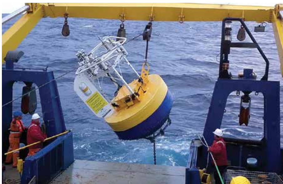
The Southern Ocean Flux Station mooring was deployed 350 nautical miles southwest of Tasmania to record meteorological and oceanographic observations to help scientists better understand climate variability. Credit: Jason Wall
