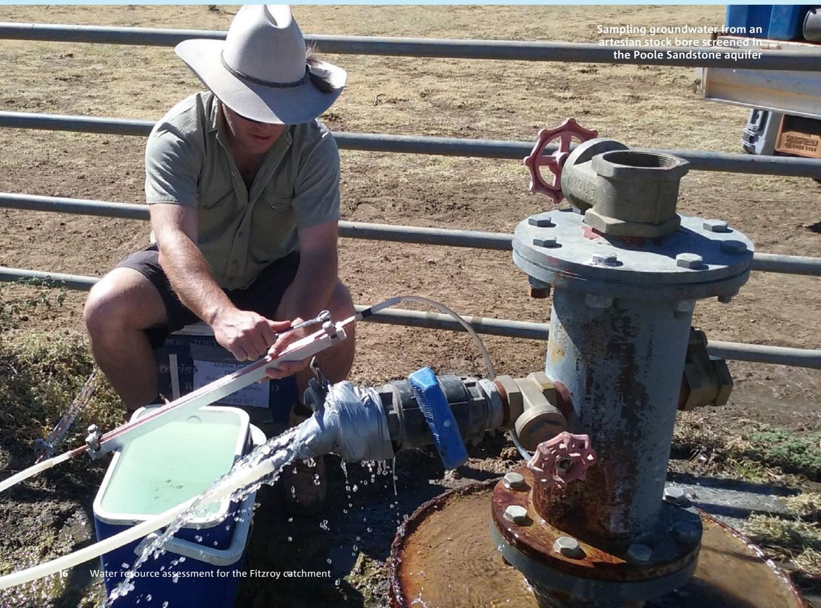
Sampling groundwater from an artesian stock bore screened in the Poole Sandstone aquifer
