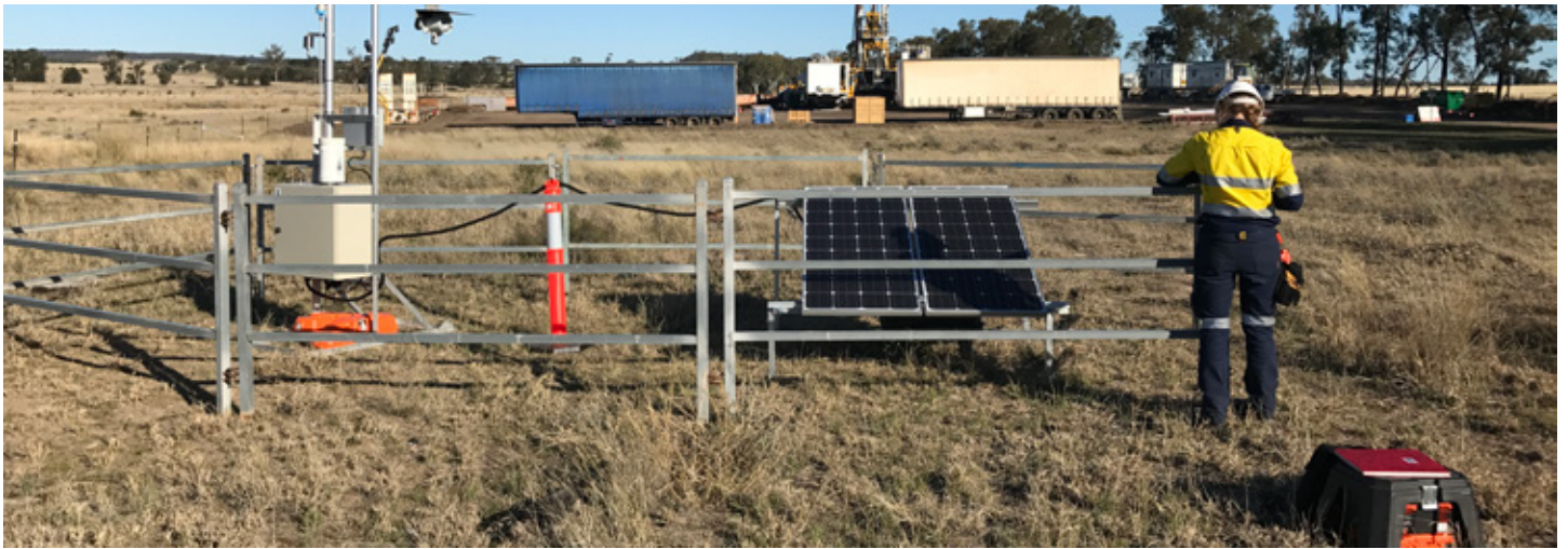
CSIRO scientist sets up a solar powered air quality monitoring station in the Surat Basin, Queensland.
