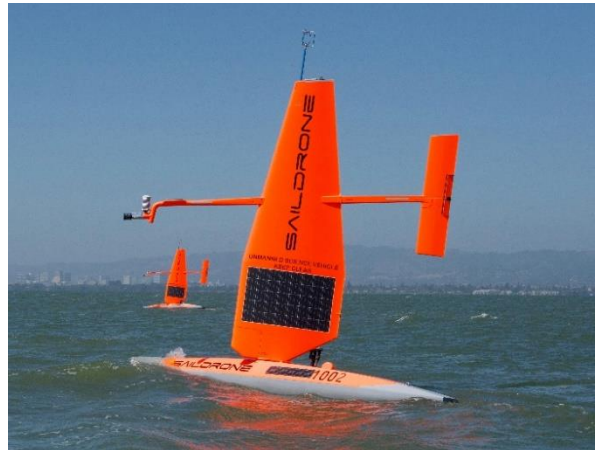
The unmanned surface vehicle, saildrone, being trialled to collect environmental data in the Gippsland region.
