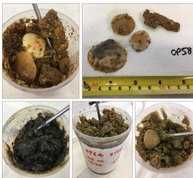
Photographs to show a representative range of sediment types collected using the Smith McIntyre grab during the FTV Bluefin survey in November 2017.
