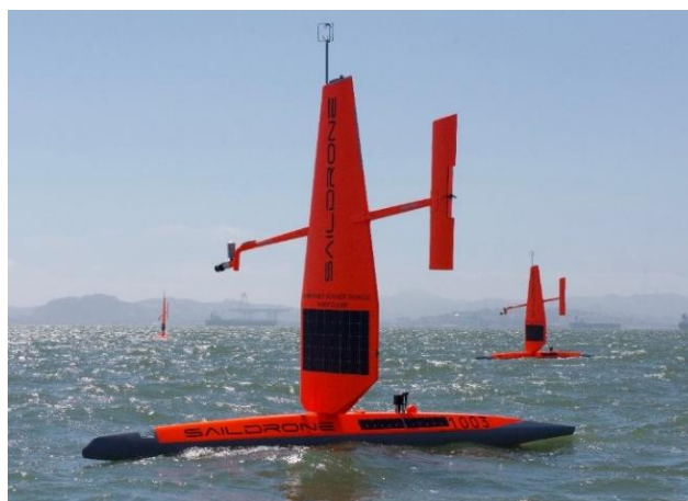
Saildrone is an unmanned surface vehicle equipped with sensor technology to measure the marine environment.
