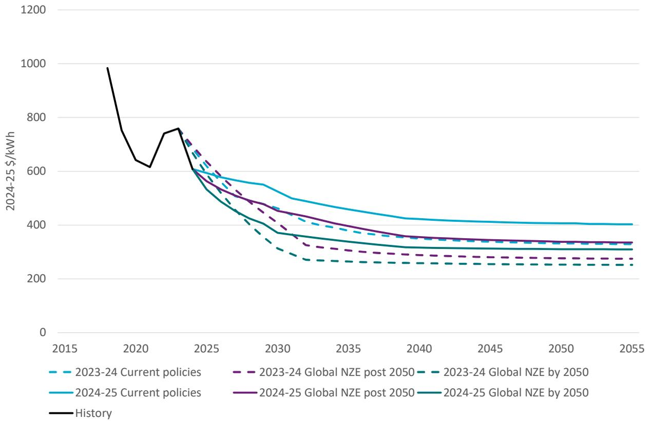
Figure 5-15 Projected total capital costs for 2-hour duration batteries by scenario (battery and balance of plant)
