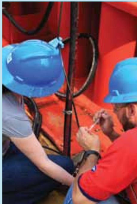
CSIRO scientists taking oil mousse samples from a water hose used on the underway hydrocarbon sensor system. Credit: Andrew Ross, CSIRO
