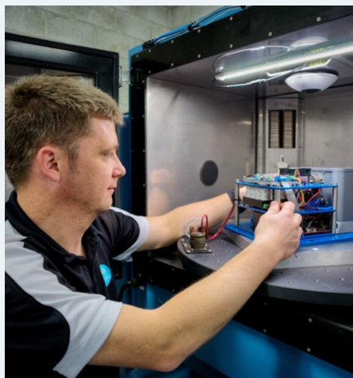
Peter Reid is calibrating and validating CSIRO's longwall guidance system electronics module before field commissioning.
