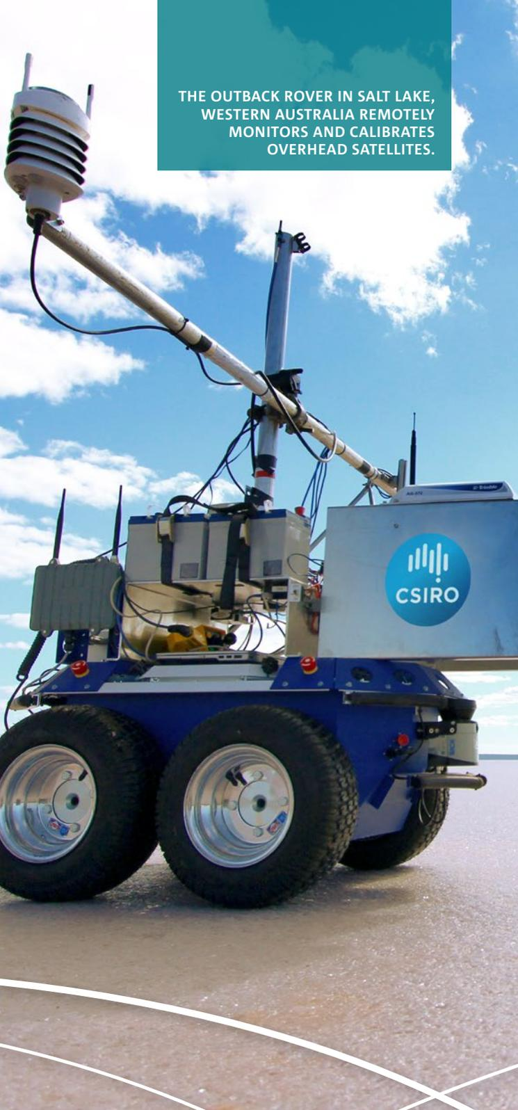
THE OUTBACK ROVER IN SALT LAKE, WESTERN AUSTRALIA REMOTELY MONITORS AND CALIBRATES OVERHEAD SATELLITES.
