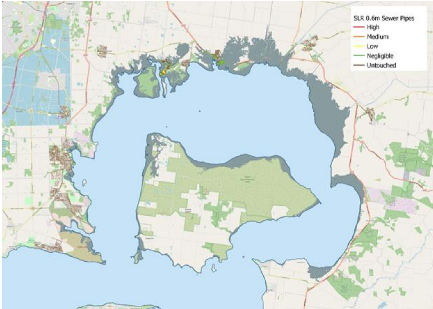
Figure 20: Infrastructure Hazard for Sewer pipes for sea level rise scenario 0.6 m. This includes a 1% AEP storm surge.
