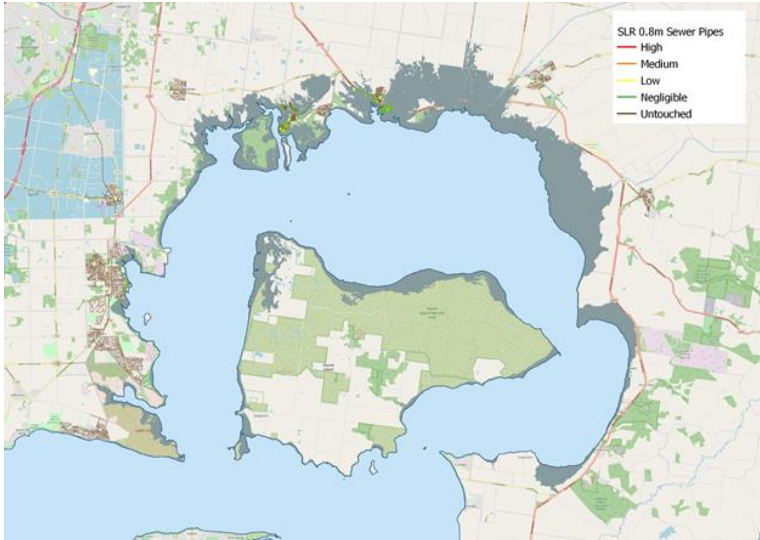
Figure 21: Infrastructure Hazard for Sewer pipes for sea level rise scenario 0.8 m. This includes a 1% AEP storm surge.
