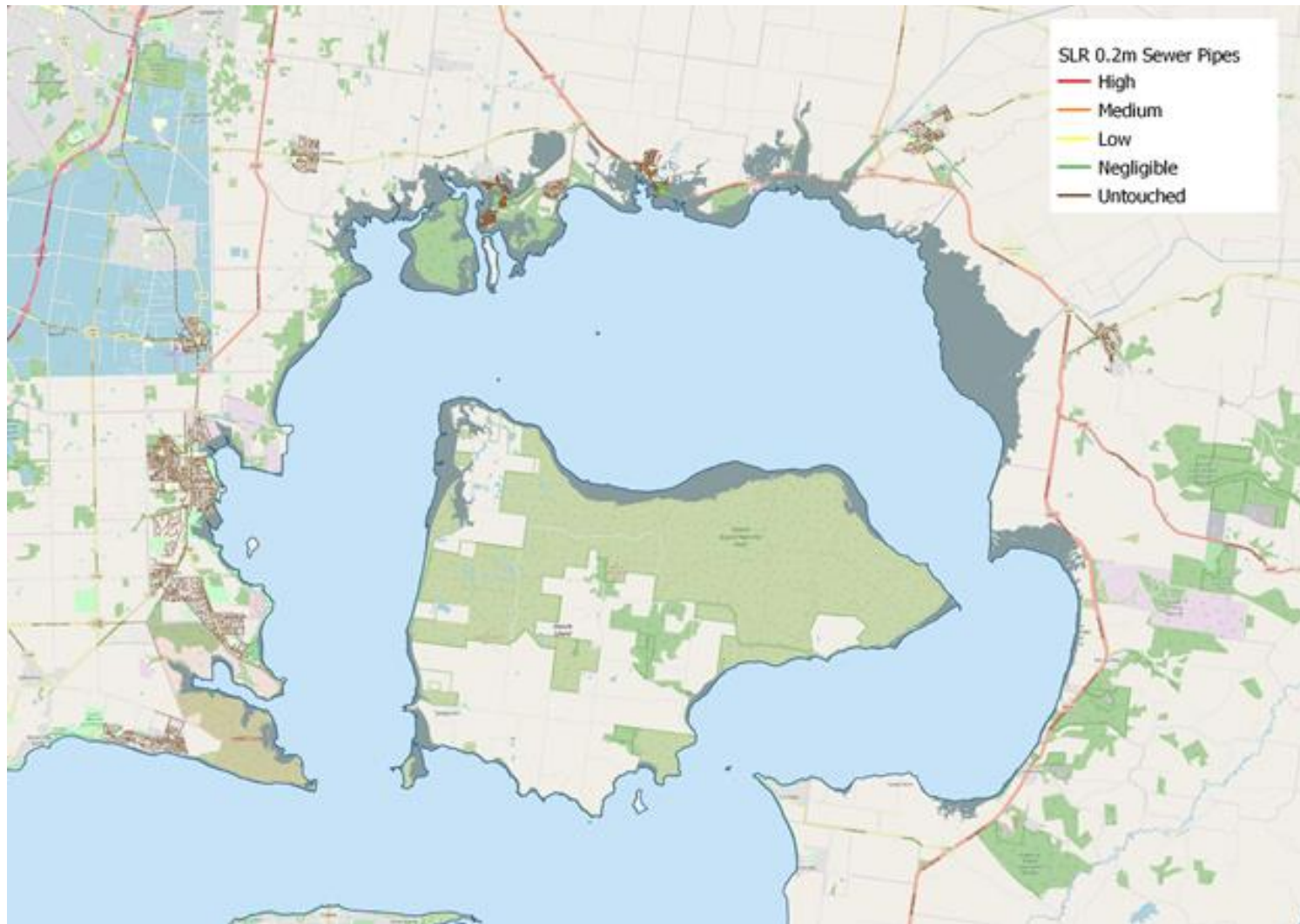
Figure 19: Infrastructure Hazard for Sewer pipes for sea level rise scenario 0.2m. This includes a 1% AEP storm surge.
