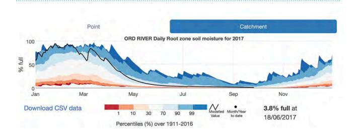
Root zone soil moisture estimates for the Ord River catchment on 18 June 2017. The Bureau's operational Australian Landscape Water Balance model simulates the flow of water through the landscape in each grid cell—entering as rainfall, passing through the vegetation and soil, and leaving through evapotranspiration, runoff or deep drainage to the groundwater.
