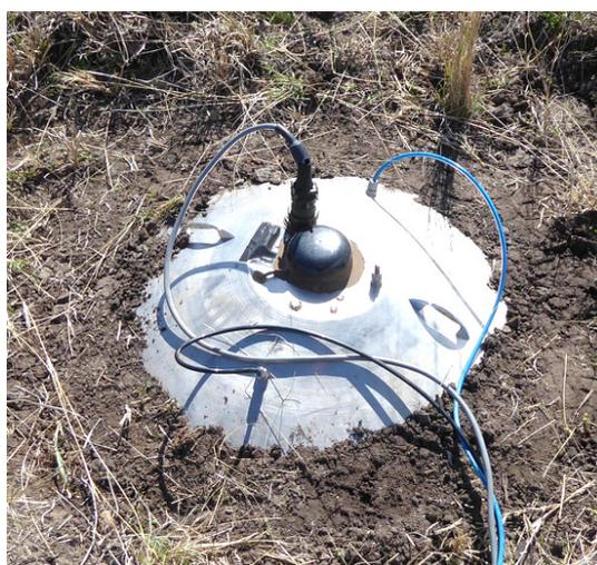
Fig.2. View of accumulation chamber during radon flux measurement
