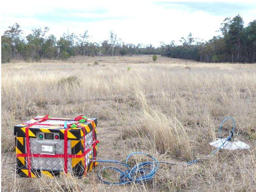
Fig.1. View of ANSTO portable radon emanometer
