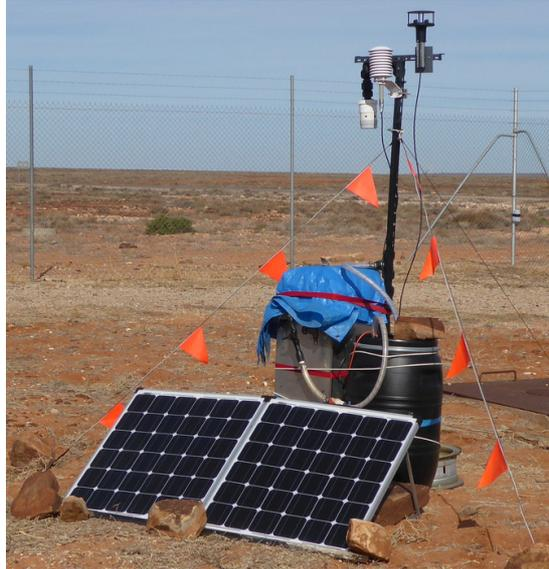
Fig.5. 100L radon detector located at survey site
