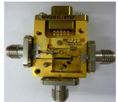
The latest CSIRO demonstrator of a compact, high-gain (40 dB) and low noise (< 0.5 dB) Ka band HTS receiver front-end module.
