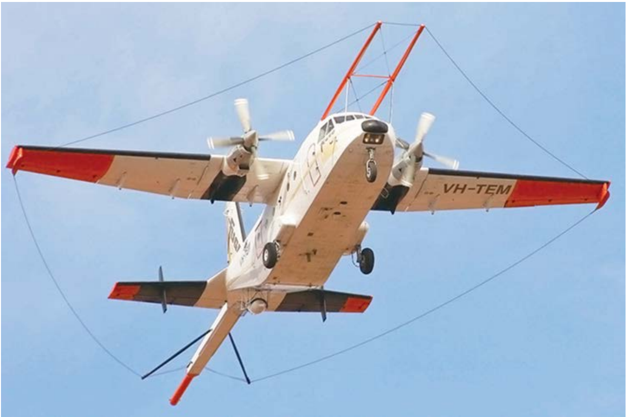
TEMPEST® AEM airborne electromagnetic acquisition system. Image credit: CGG Airborne.
