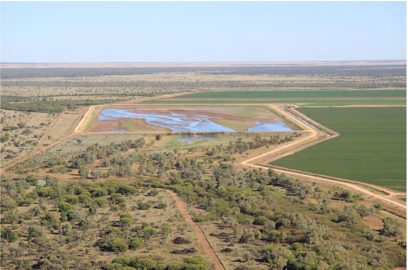
**Figure 3-1 Rectangular ringtank in the Flinders catchment, Queensland**
