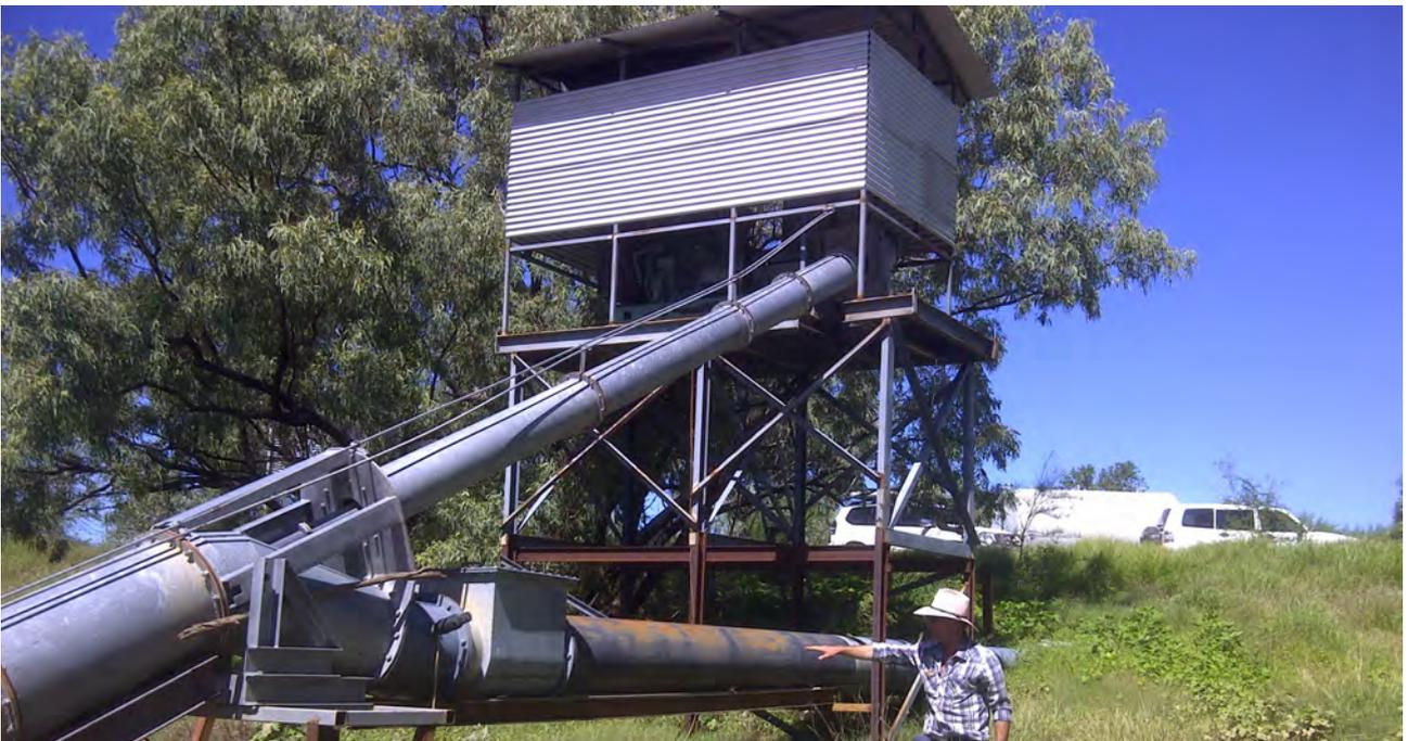
**Figure 3-2 Diesel powered axial-flow flood-harvesting pump in Flinders catchment, Queensland**
