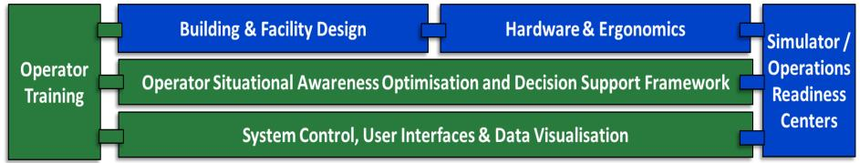
Figure 2-6 The six CROF pillars as defined for the CROF model associated with human factors and operator interaction with the software systems and data in the control room.
