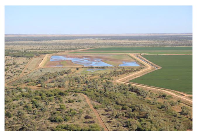
**Figure 3-1 Rectangular ringtank in the Flinders catchment, Queensland** Photo: CSIRO.
