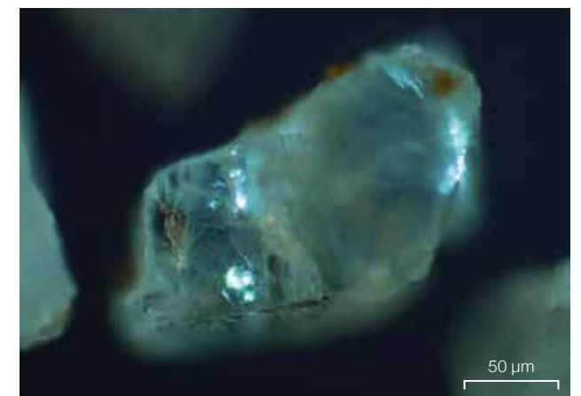
Above: Fluid inclusion methodologies identified traces of oil in sediments, such as sand, as well as analysing their geochemical characteristics and entrapment history.
