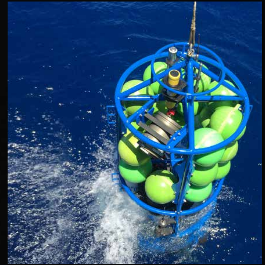
Right: A profiling multi-frequency acoustic and optical system was used to detect and quantify micronekton (small fish, squids, crustaceans and larger gelatinous organisms, such as the siphonophore, Praya reticulata shown on the left).
